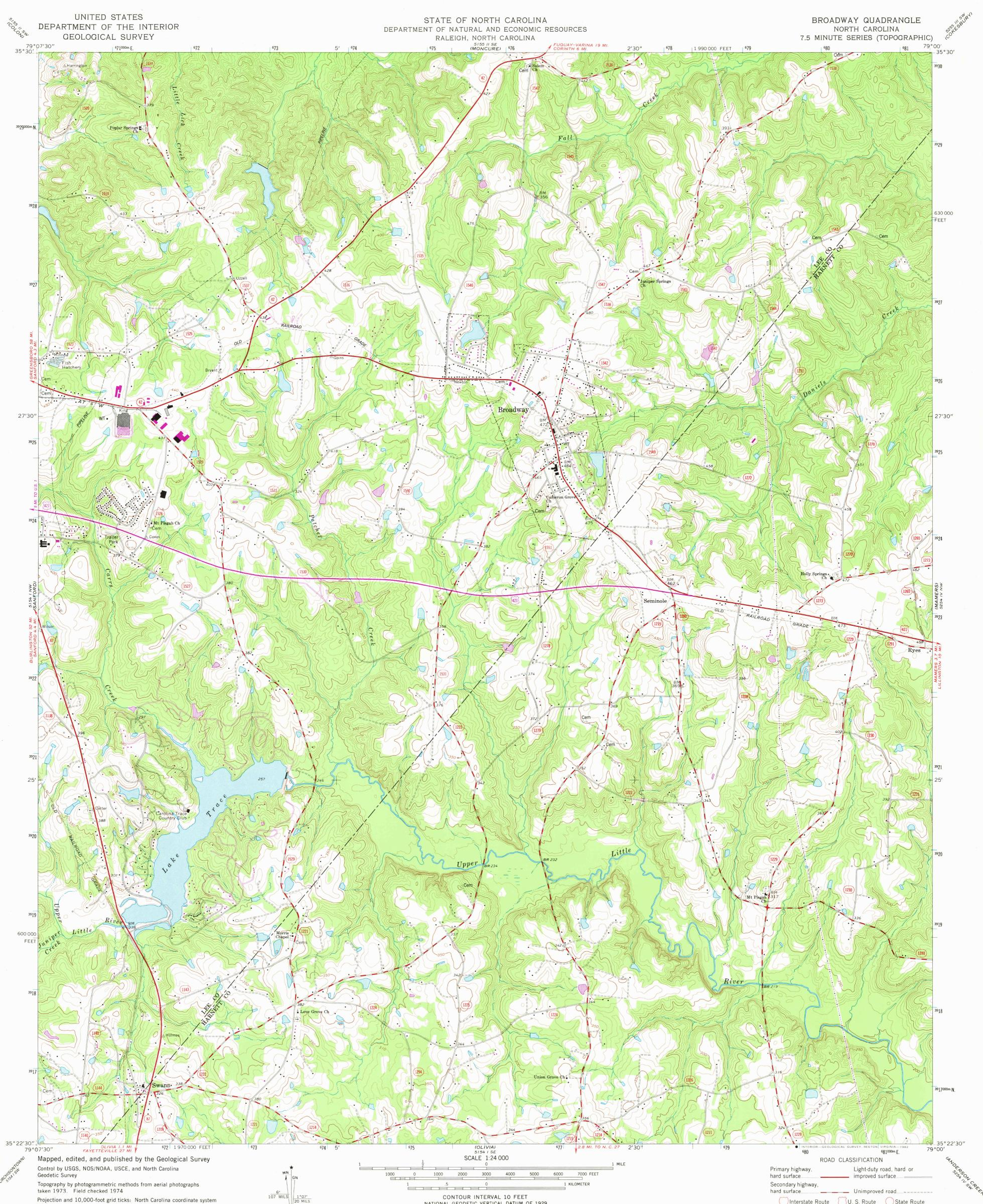
Projection and 10,000-foot grid ticks: North Carolina coordinate system (Lambert conformal conic). 1000-meter Universal Transverse Mercator grid ticks, zone 17, shown in blue. 1927 North American Datum To place on the predicted North American Datum 1983 move the projection lines 12 meters south and 22 meters west as shown by dashed corner ticks
