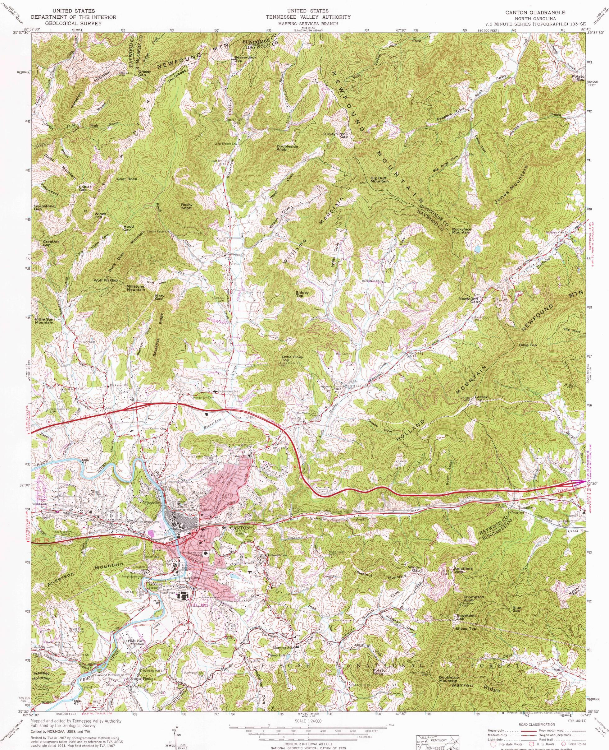
Polyconic projection. 1927 North American Datum To place on the predicted North American Datum 1983 move the projection lines 8 meters south and 12 meters west as shown by dashed corner ticks 10,000 foot grid based on North Carolina rectangular coordinate system 1000 meter Universal Transverse Mercator grid ticks, zone 17, shown in blue
