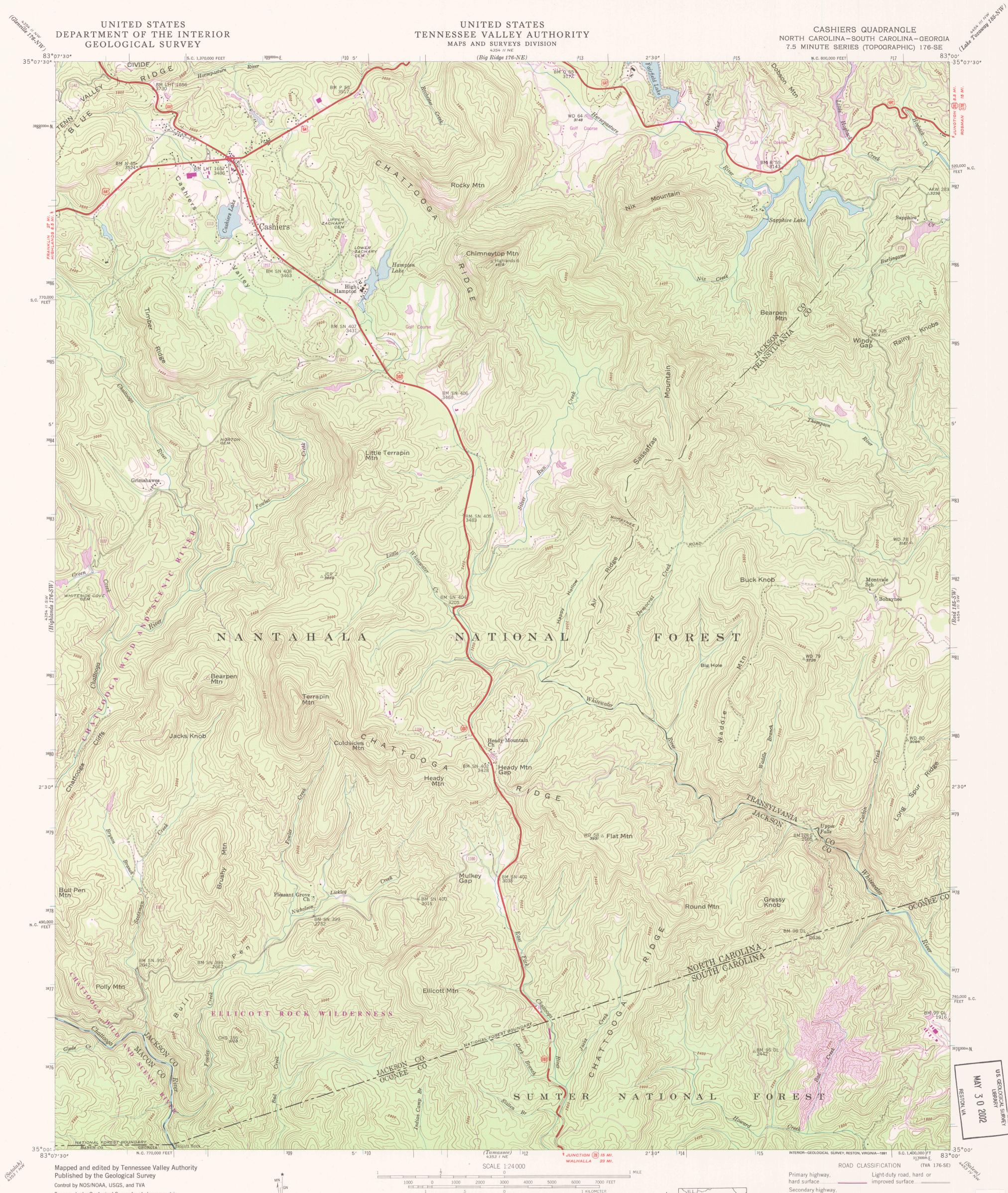
Topography by Geological Survey by photogrammetric methods. Field checked by Tennessee Valley Authority 1946 Polyconic projection. 1927 North American Datum 10,000-foot grid ticks based on North Carolina coordinate system and South Carolina coordinate system, north zone 1000-meter Universal Transverse Mercator grid ticks, zone 17, shown in blue To place on the predicted North American Datum 1983 move the projection lines 9 meters south and 11 meters west as shown by dashed corner ticks
