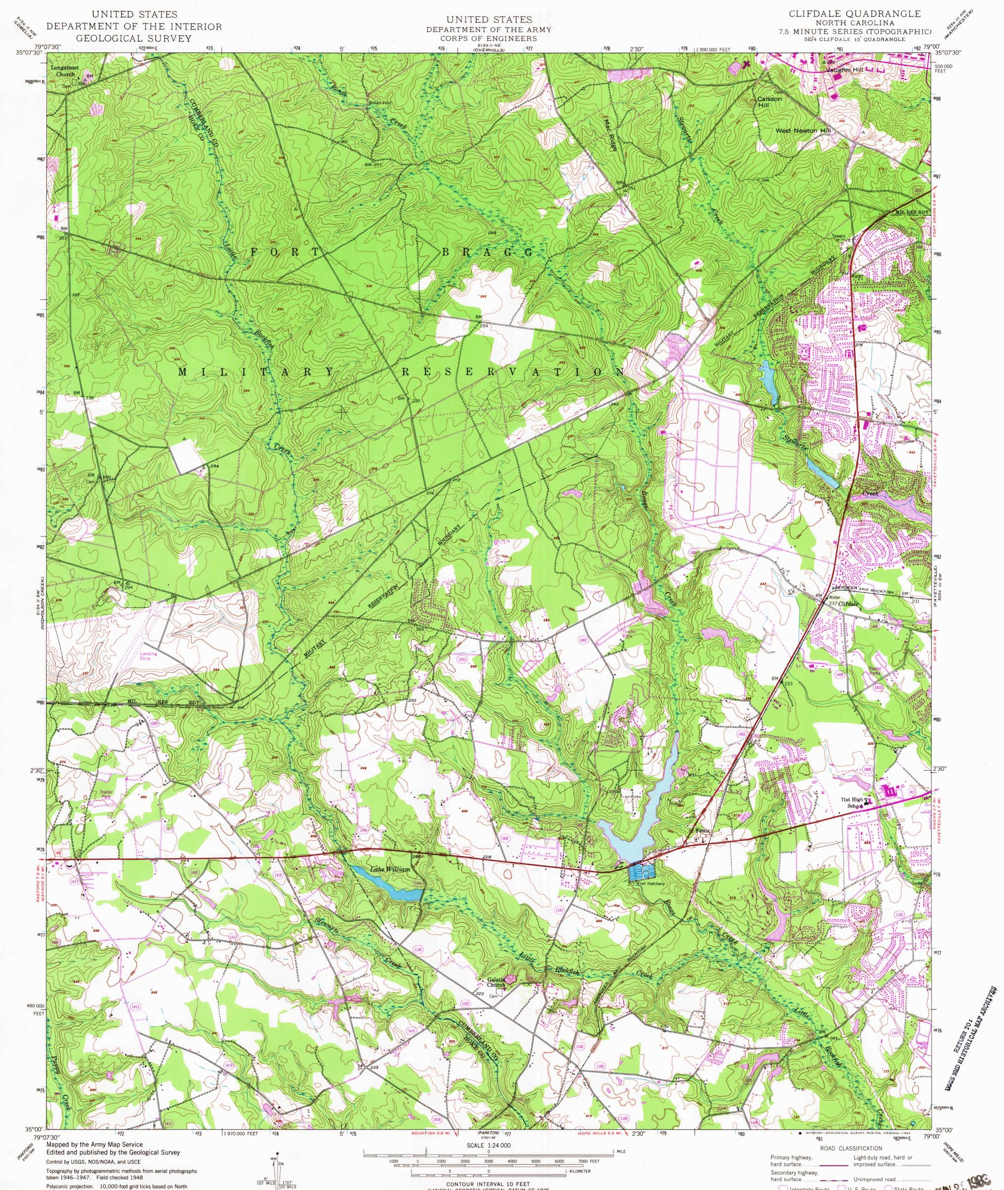
Polyconic projection. 10,000-foot grid ticks based on North Carolina coordinate system. 1000-meter Universal Transverse Mercator grid ticks, zone 17, shown in blue. 1927 North American Datum. To place on the predicted North American Datum 1983 move the projection lines 12 meters south and 22 meters west as shown by dashed corner ticks
