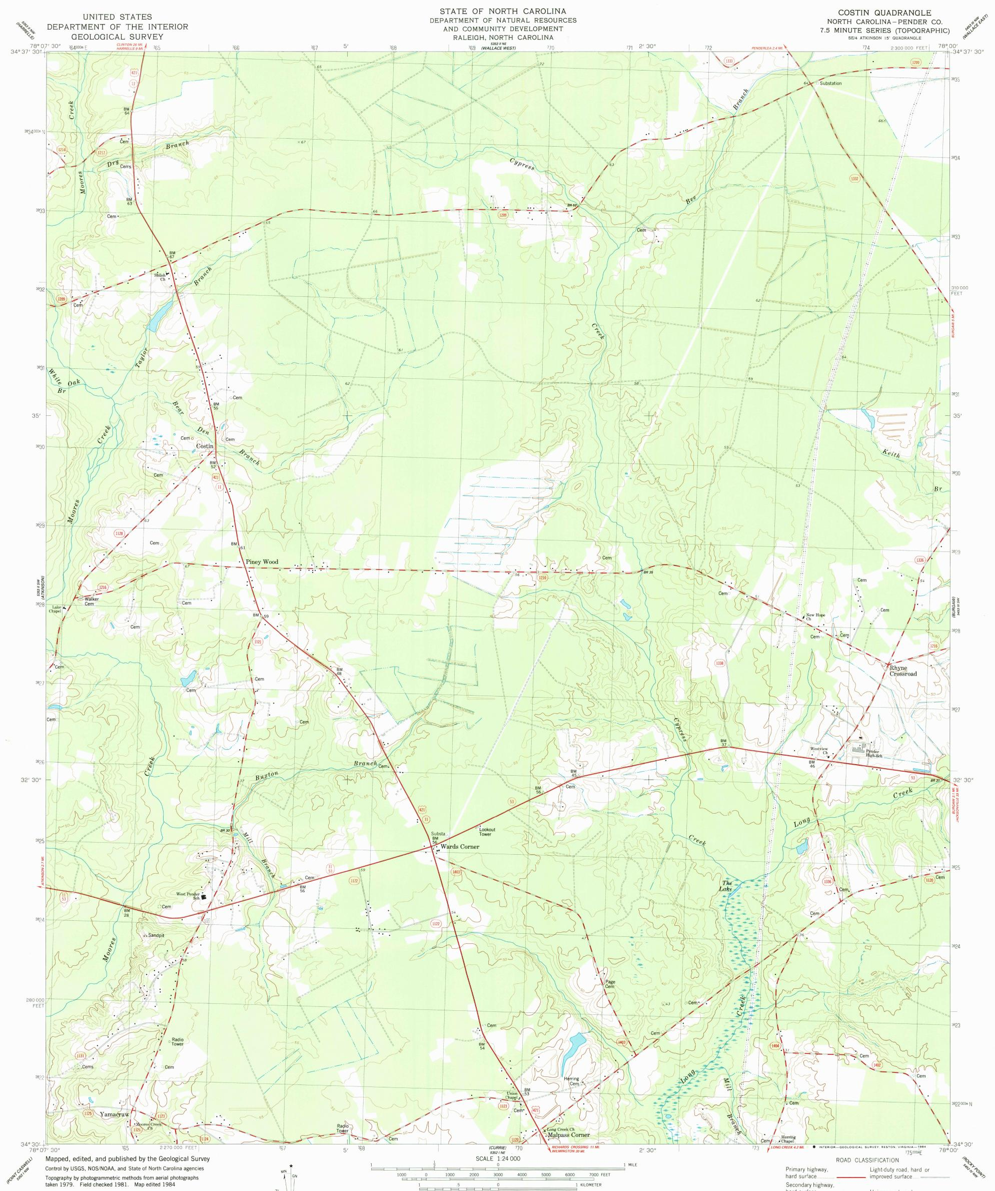
Projection and 1000-meter grid, zone 17: Universal Transverse Mercator 10,000-foot grid ticks based on North Carolina coordinate system 1927 North American Datum To place on the predicted North American Datum 1983 move the projection lines 14 meters south and 25 meters west as shown by dashed corner ticks  $\frac{7^{\circ}}{124 \text{ MILS}} \sqrt{\frac{1^{\circ}40'}{30 \text{ MILS}}}$
