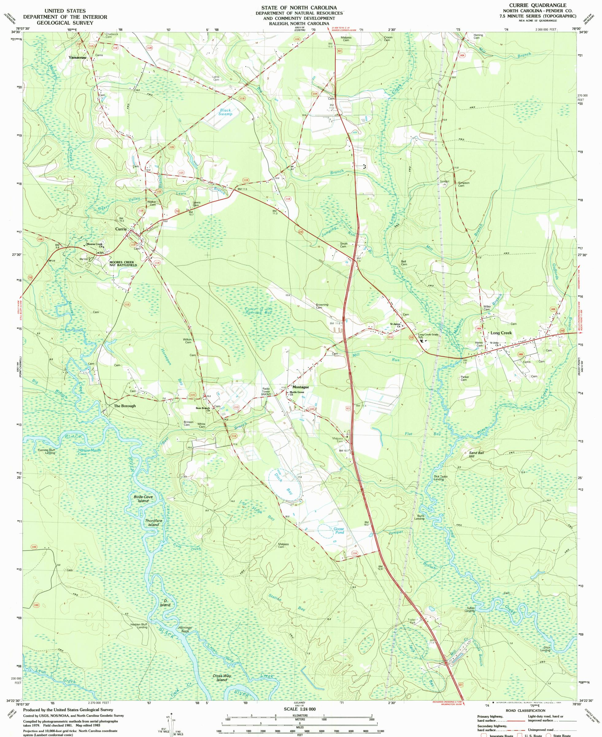
Projection and 10,000-foot grid ticks: North Carolina coordinate system (Lambert conformal conic) 1000-meter Universal Transverse Mercator grid, zone 17 1927 North American Datum To place on the predicted North American Datum 1983 move the projection lines 14 meters south and 25 meters west as shown by dashed corner ticks
