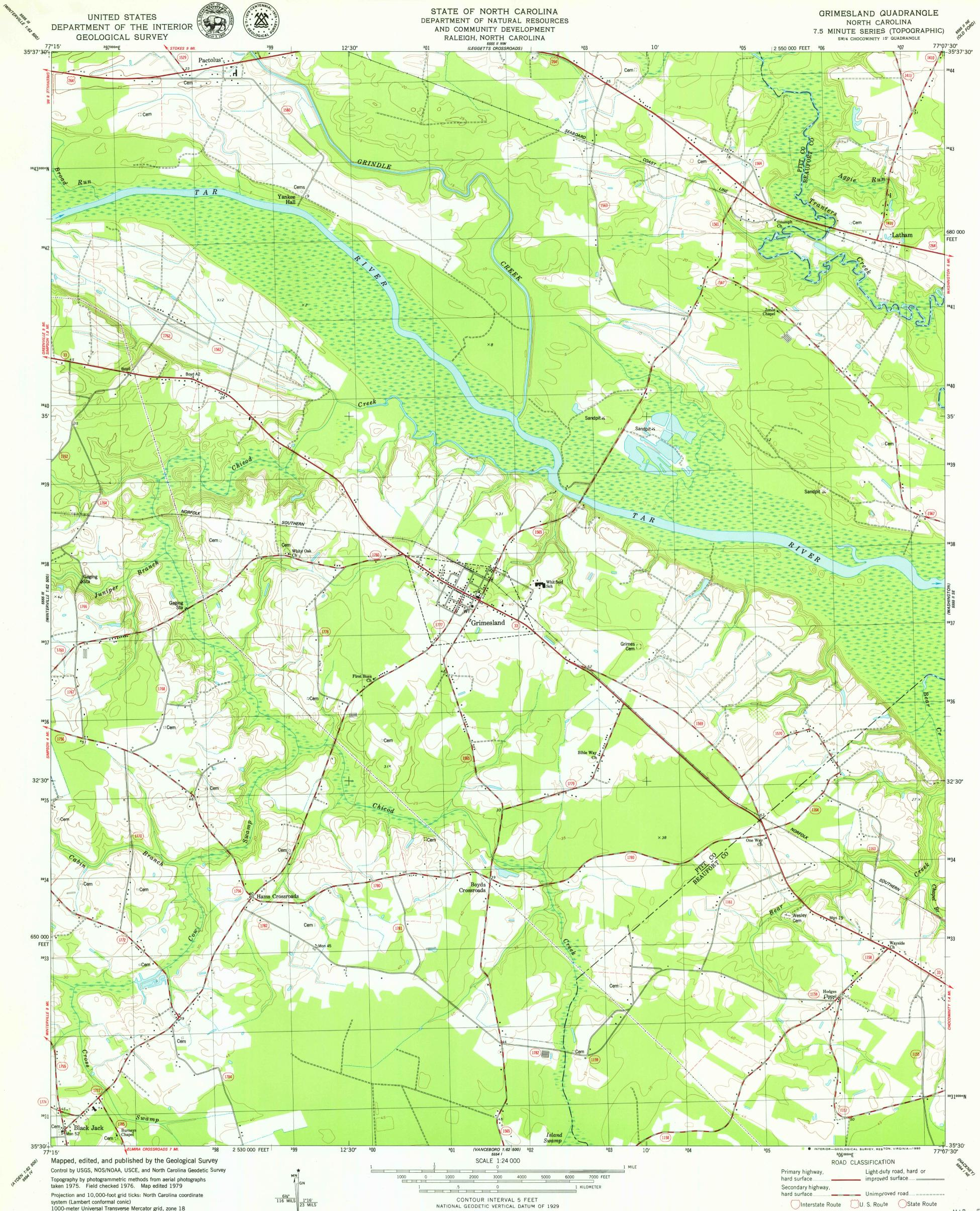
1000-meter Universal Transverse Mercator grid, zone 18 1927 North American Datum To place on the predicted North American Datum 1983 move the projection lines 12 meters south and 27 meters west as shown by dashed corner ticks
