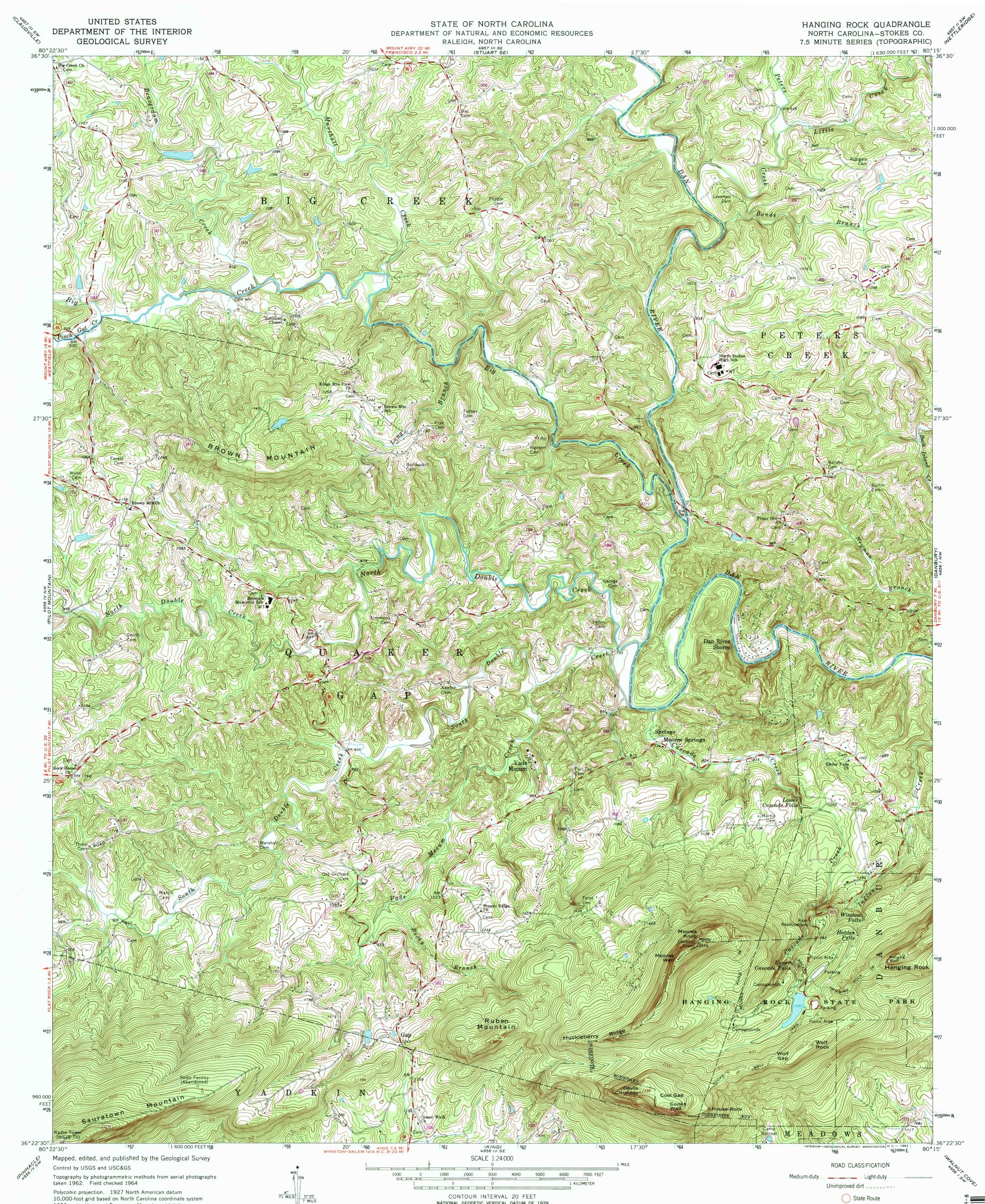
10,000-foot grid based on North Carolina coordinate system 1000-meter Universal Transverse Mercator grid ticks, zone 17, shown in blue The difference between 1927 North American Datum and North American Datum of 1983 (NAD 83) for 7.5-minute intersections is given in USGS Bulletin 1875. The NAD 83 is shown by dashed corner ticks Revisions shown in purple compiled from aerial photographs taken 1971. This information not field checked
