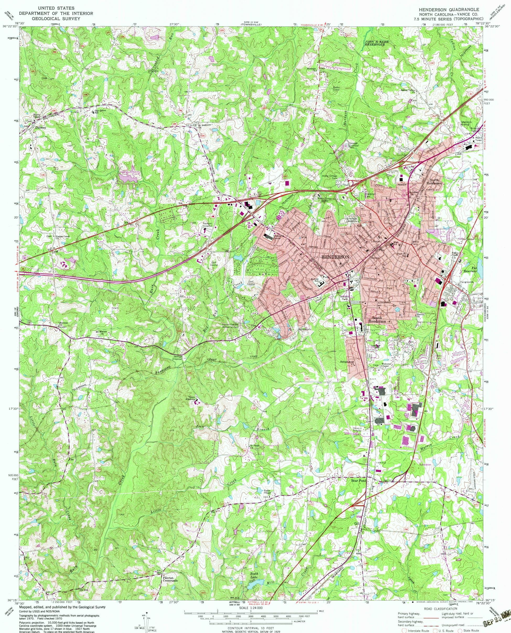
Carolina coordinate system. 1000-meter Universal Transverse Mercator grid ticks, zone 17 shown in blue. 1927 North American Datum. To place on the predicted North American Datum 1983 move the projection lines 12 meters south and 24 meters west as shown by dashed corner ticks
