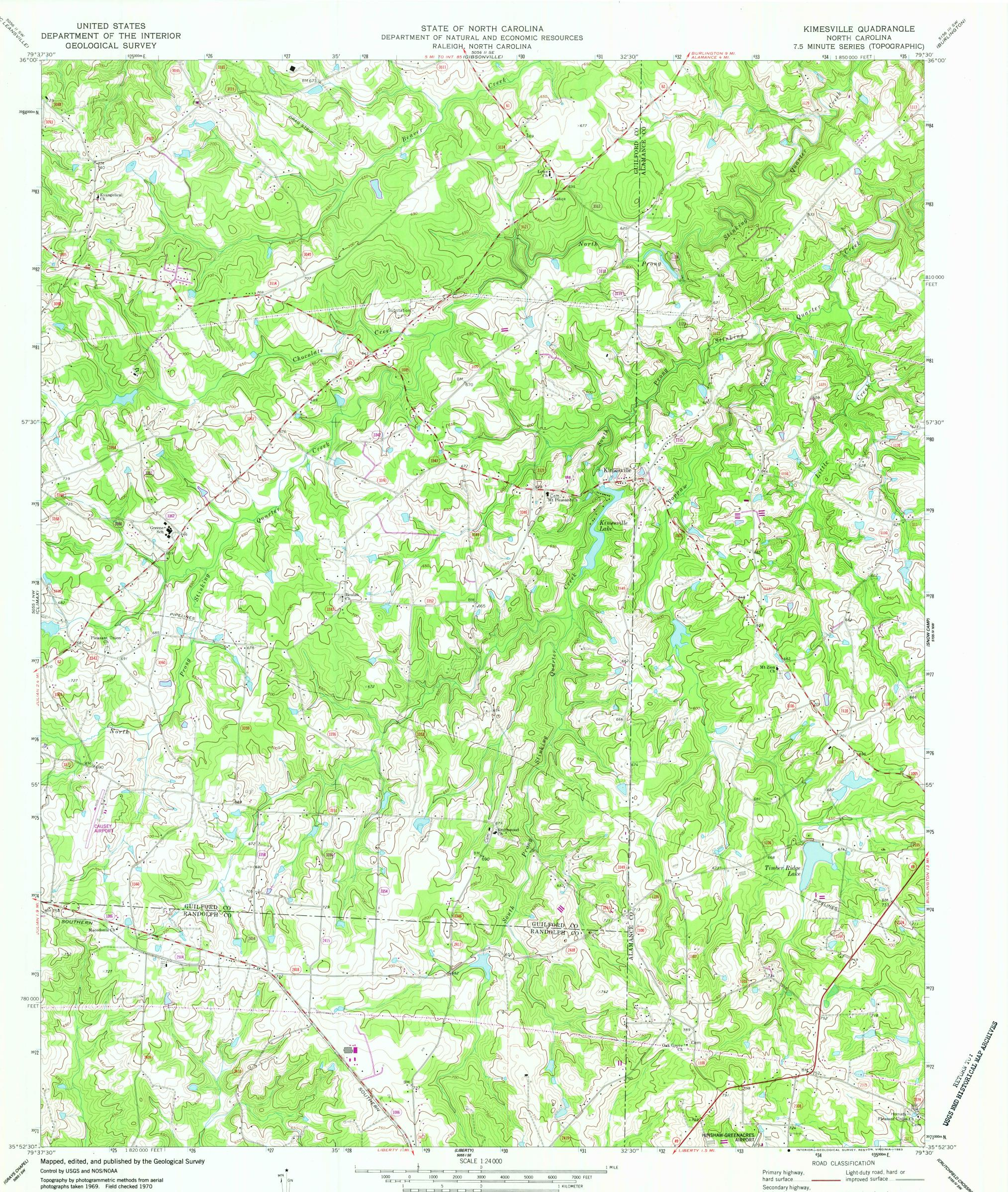
Polyconic projection. 10,000-foot grid ticks based on North Carolina coordinate system. 1000-meter Universal Transverse Mercator grid ticks, zone 17, shown in blue. 1927 North American Datum. To place on the predicted North American Datum 1983 move the projection lines 11 meters south and 20 meters west as shown by dashed corner ticks
