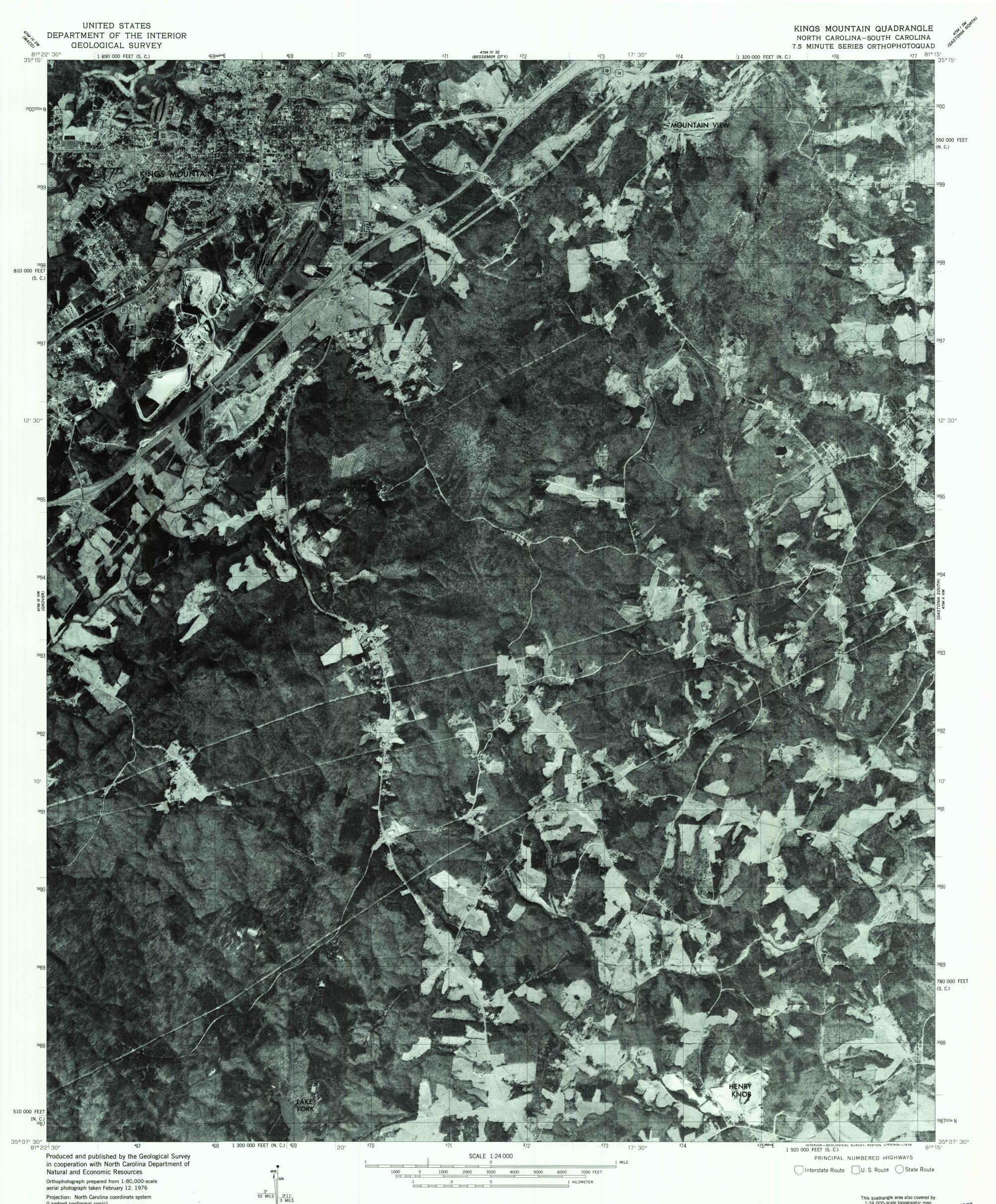
Projection: North Carolina coordinate system (Lambert conformal conic) 10,000-foot grid ticks based on North Carolina coordinate system, and South Carolina coordinate system, north zone 1000-meter Universal Transverse Mercator grid, zone 17. 1927 North American datum
