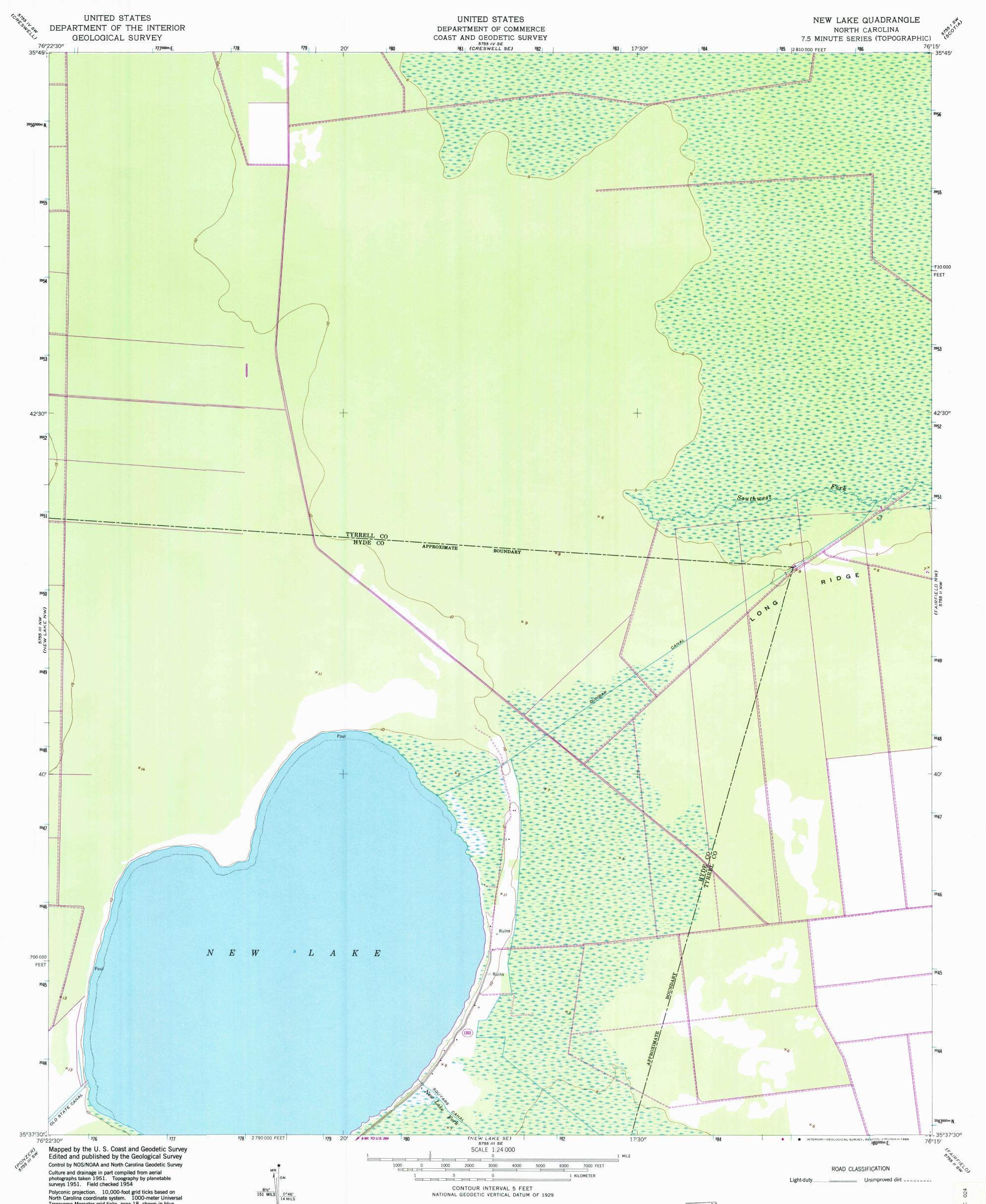
Polyconic projection. 10,000-foot grid ticks based on North Carolina coordinate system. 1000-meter Universal Transverse Mercator grid ticks, zone 18, shown in blue 1927 North American Datum To place on the predicted North American Datum 1983 move the projection lines 12 meters south and 29 meters west as shown by dashed corner ticks west as shown by dashed corner ticks
