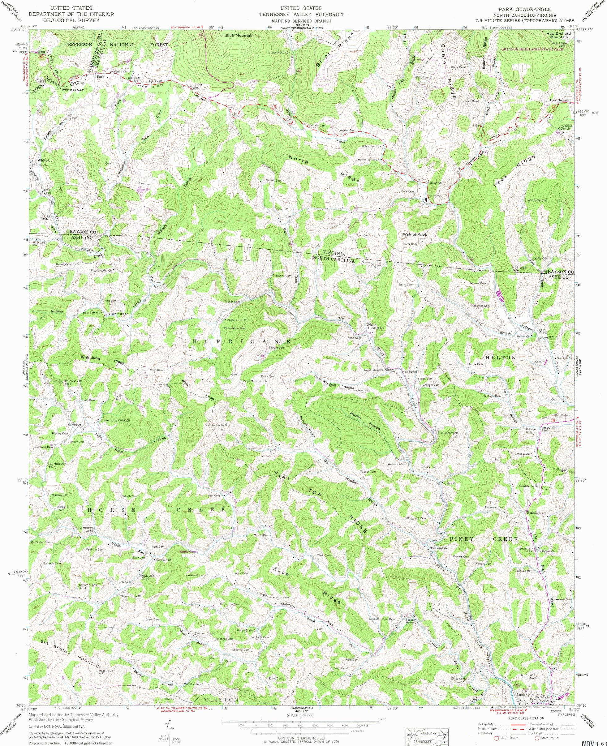
Polyconic projection. 10,000-foot grid ticks based on North Carolina and Virginia (south) rectangular coordinate systems 1000-meter Universal Transverse Mercator grid ticks, zone 17, shown in blue. 1927 North American Datum To place on the predicted North American Datum 1983 move the projection lines 8 meters south and 15 meters west as shown by dashed corner ticks
