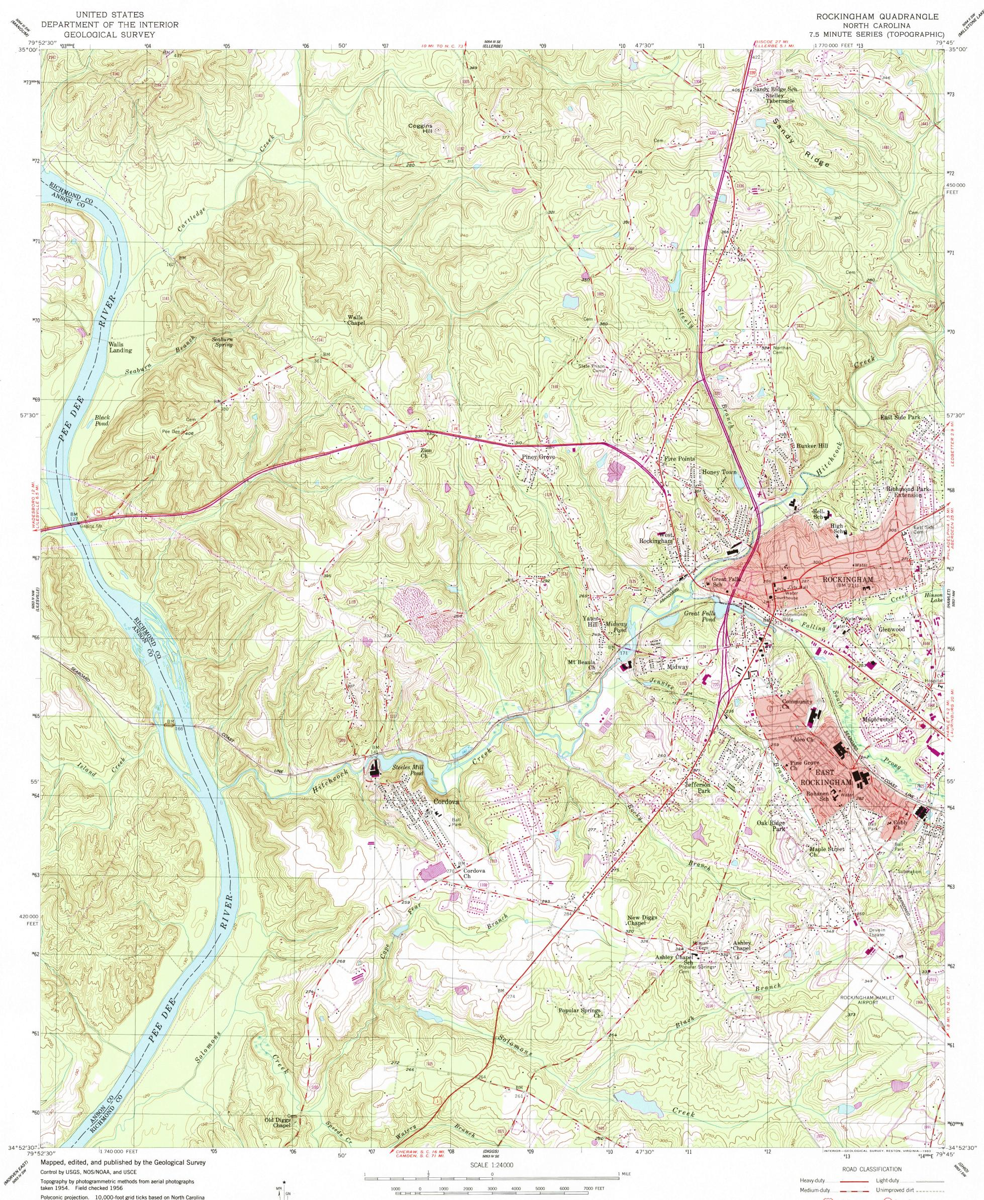
coordinate system. 1000-meter Universal Transverse Mercator grid, zone 17. 1927 North American Datum. To place on the predicted North American Datum 1983 move the projection lines 12 meters south and 20 meters west as shown by dashed corner ticks
