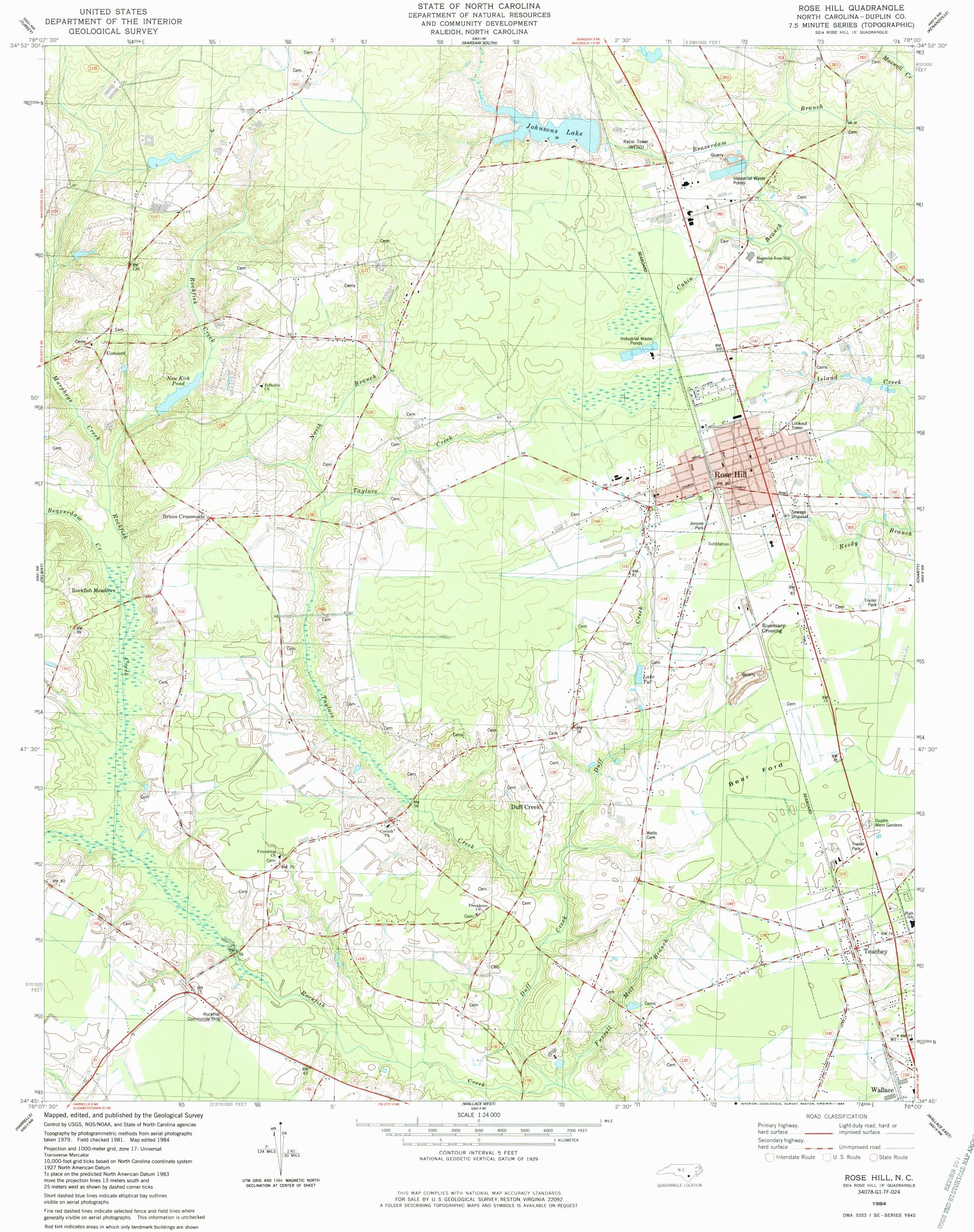
Transverse Mercator 10,000-foot grid ticks based on North Carolina coordinate system 1927 North American Datum To place on the predicted North American Datum 1983 move the projection lines 13 meters south and 25 meters west as shown by dashed corner ticks
