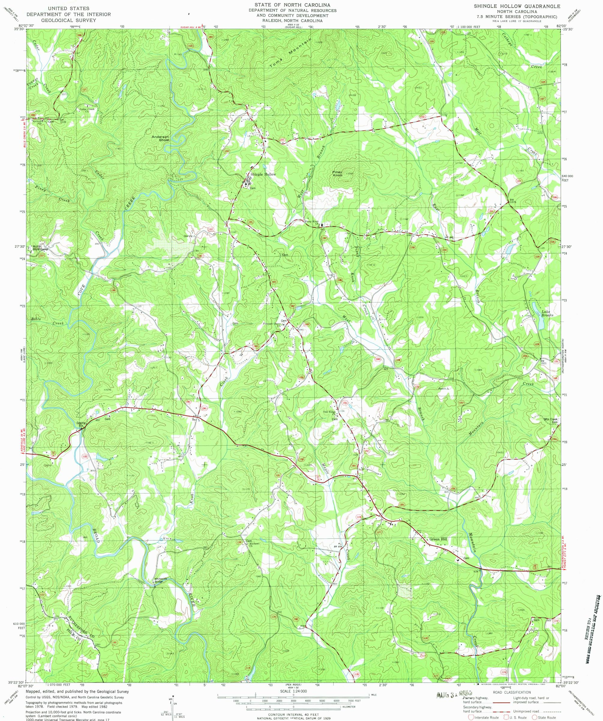
1000-meter Universal Transverse Mercator grid, zone 17 1927 North American Datum To place on the predicted North American Datum 1983 move the projection lines 9 meters south and 14 meters west as shown by dashed corner ticks
