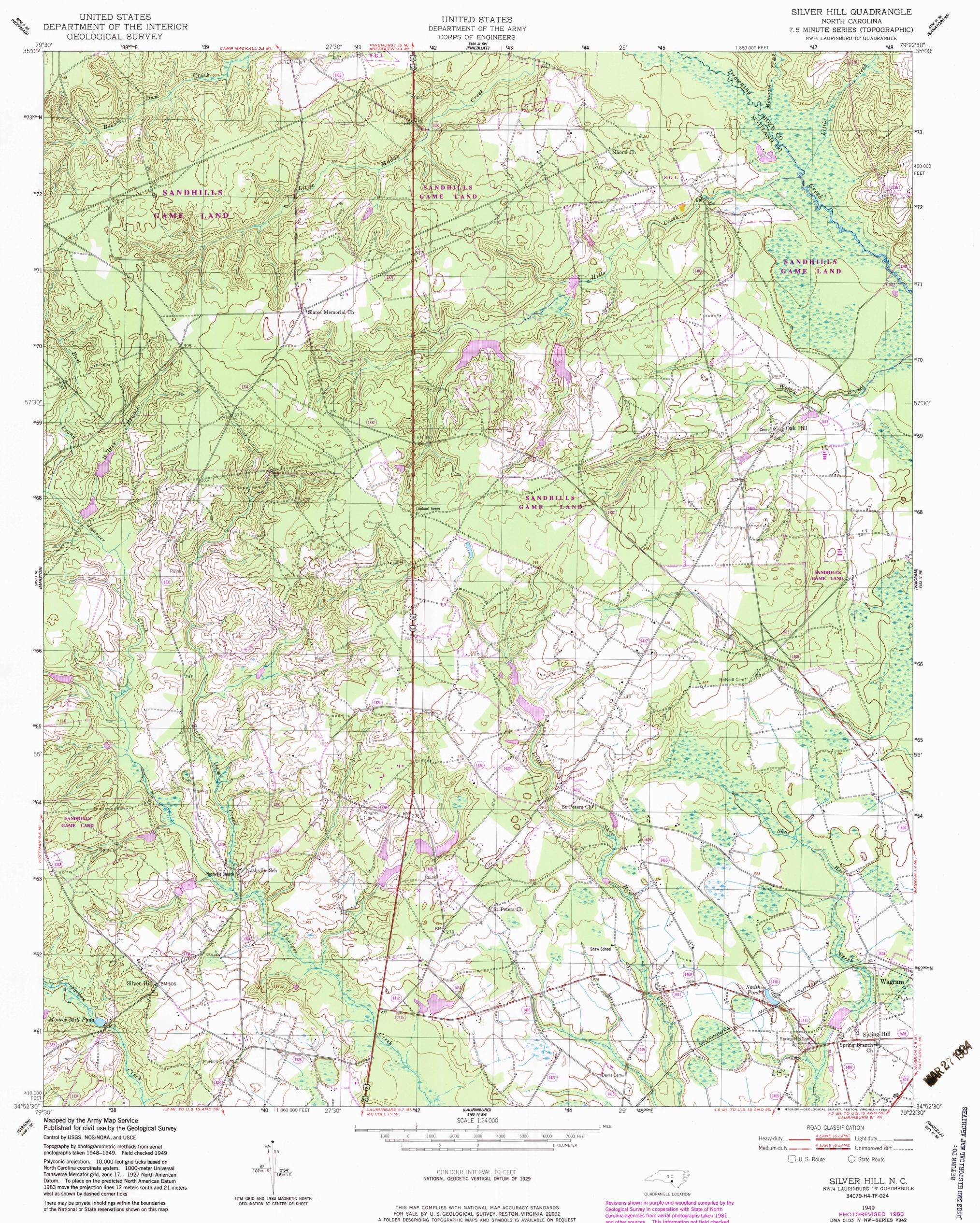
Polyconic projection. 10,000-foot grid ticks based on North Carolina coordinate system. 1000-meter Universal Transverse Mercator grid, zone 17. 1927 North American Datum. To place on the predicted North American Datum 1983 move the projection lines 12 meters south and 21 meters west as shown by dashed corner ticks
