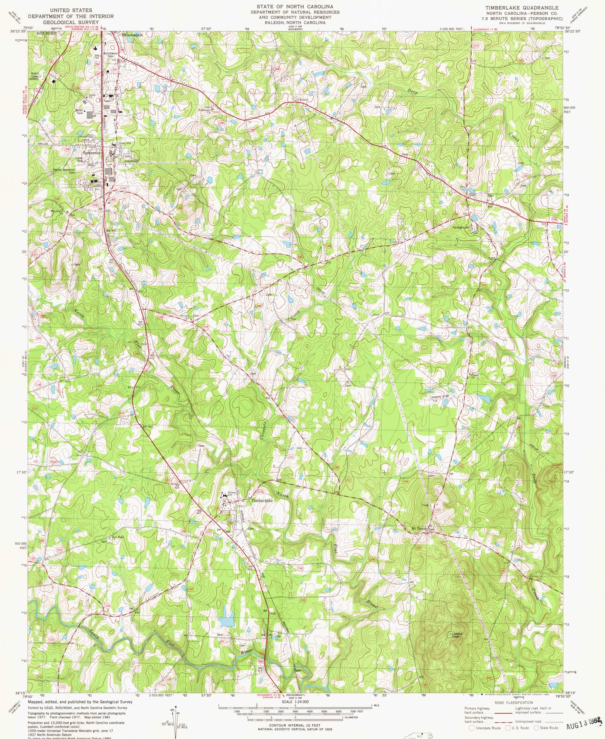
1000-meter Universal Transverse Mercator grid, zone 17 1927 North American Datum To place on the predicted North American Datum 1983 move the projection lines 11 meters south and 22 meters west as shown by dashed corner ticks
