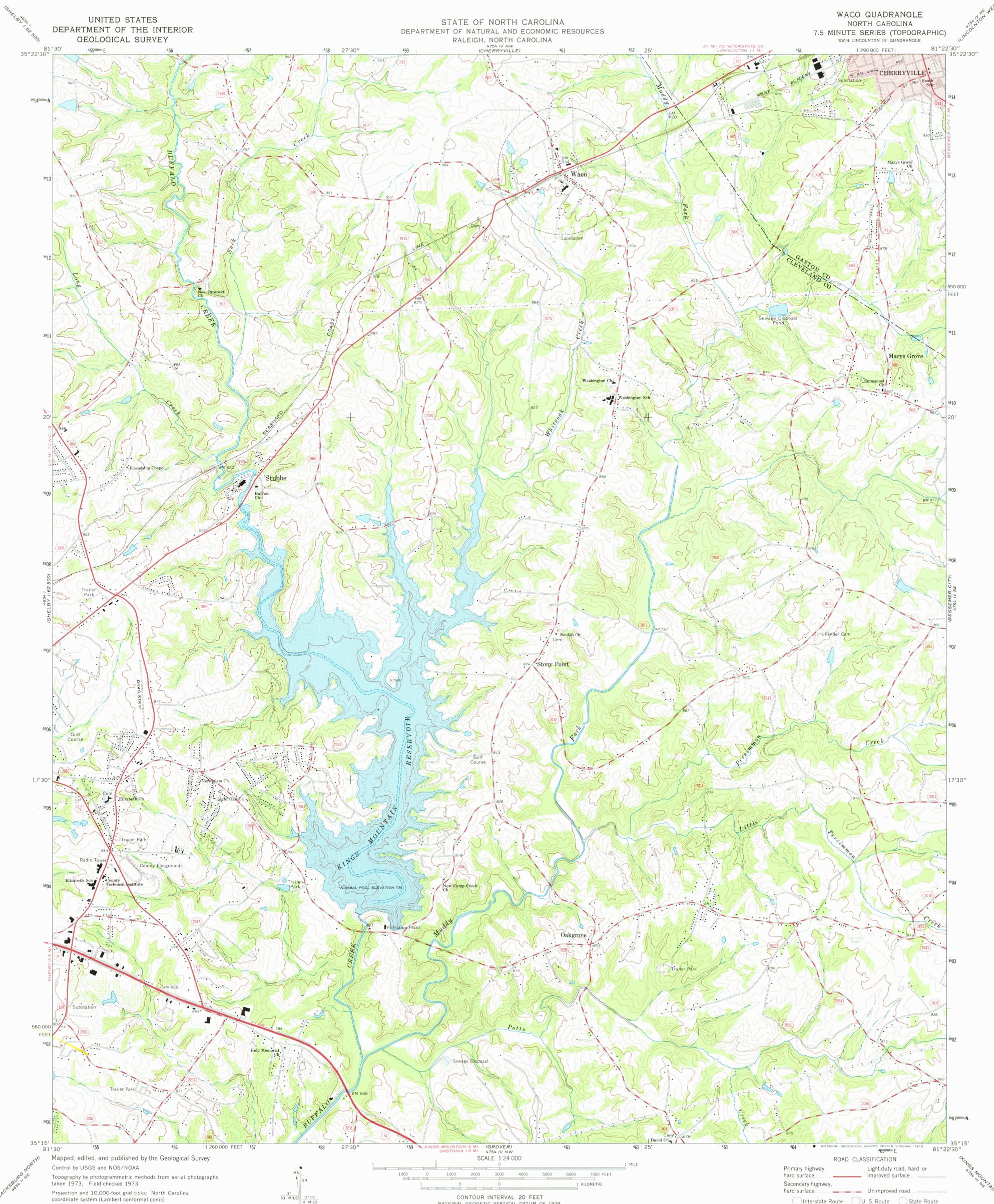
coordinate system (Lambert conformal conic) 1000-metre Universal Transverse Mercator grid ticks, zone 17, shown in blue. 1927 North American datum
