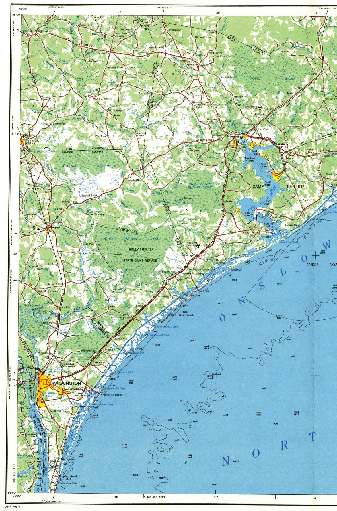
Prepared by the Army Map Service (AM), Corps of Engineers, U. S. Army, Washington, D. C. Compiled in 1954 from: North Carolina, 1:24,000, USGS, 1950-51; North Carolina, 1:50,000, AMS, 1948; USC&GS Charts, 1938-47; County Highway Maps 1948-49. Planimetric detail revised by photo-planimetric methods. Control by USC&GS. Map field checked, 1953.
