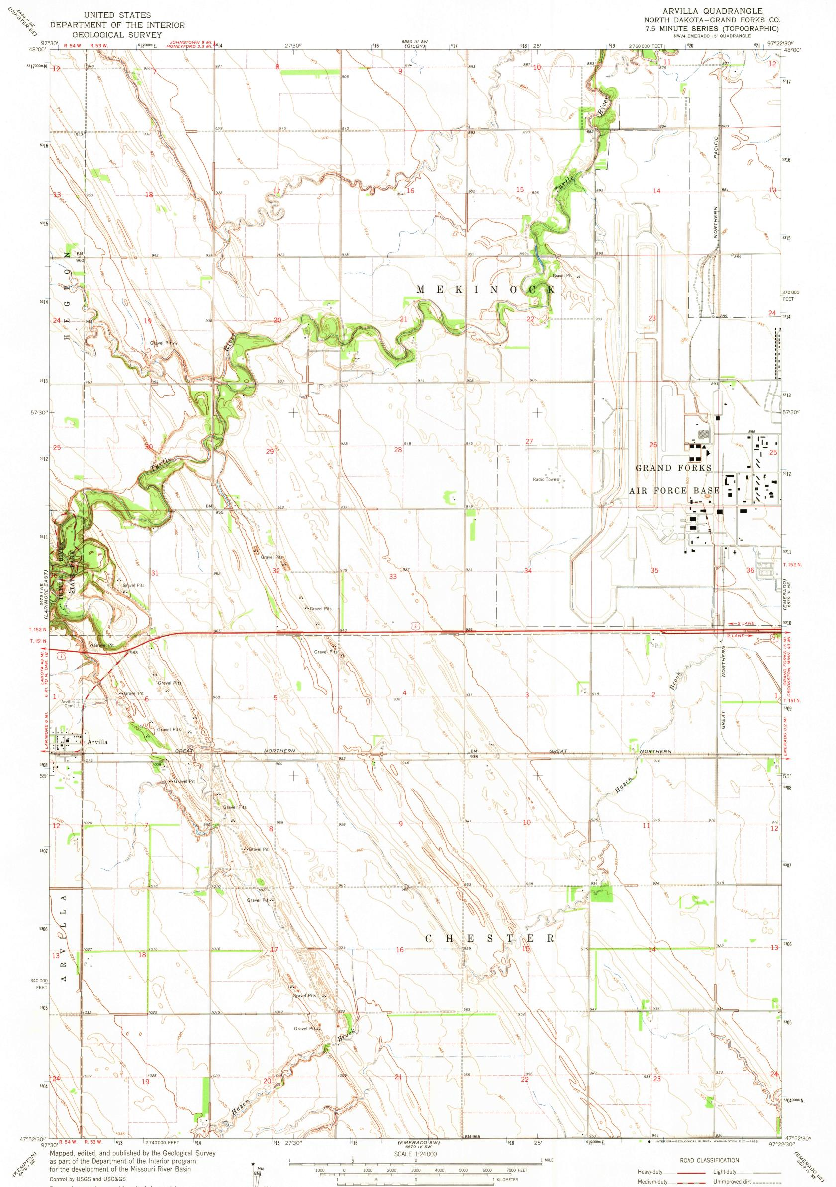
Topography by photogrammetric methods from aerial photographs taken 1961 and planetable surveys 1963
