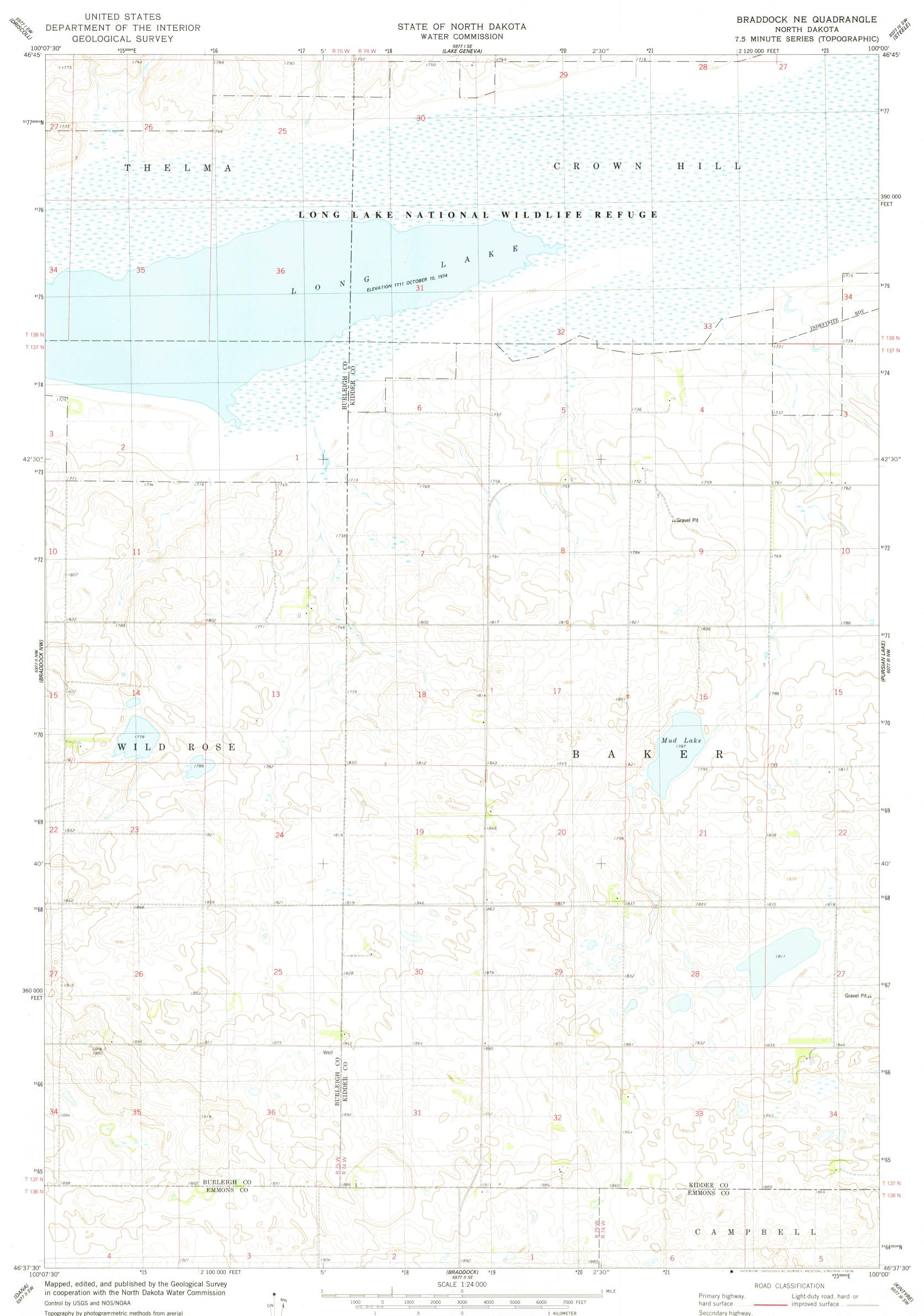
Topography by photogrammetric methods from arerial photographs taken 1974. Field checked 1975 Projection and 10,000-foot grid ticks: North Dakota coordinate system, south zone (Lambert conformal conic) 1000-meter Universal Transverse Mercator grid, zone 14. 1927 North American datum Fine red dashed lines indicate selected fence and field lines where generally visible on aerial photographs This information is unchecked
