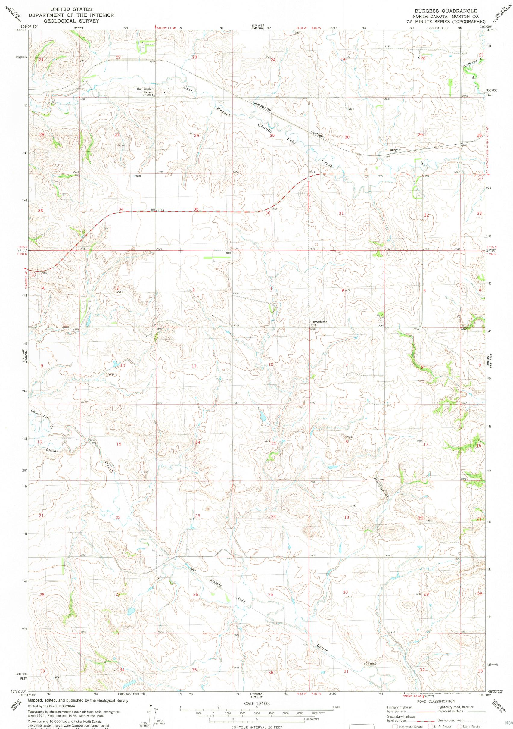
Projection and 10,000-foot grid ticks: North Dakota coordinate system, south zone (Lambert conformal conic) 1000-meter Universal Transverse Mercator grid, zone 14 1927 North American datum To place on the predicted North American Datum 1983 move the projection lines 5 meters north and 35 meters east as shown by dashed corner ticks
