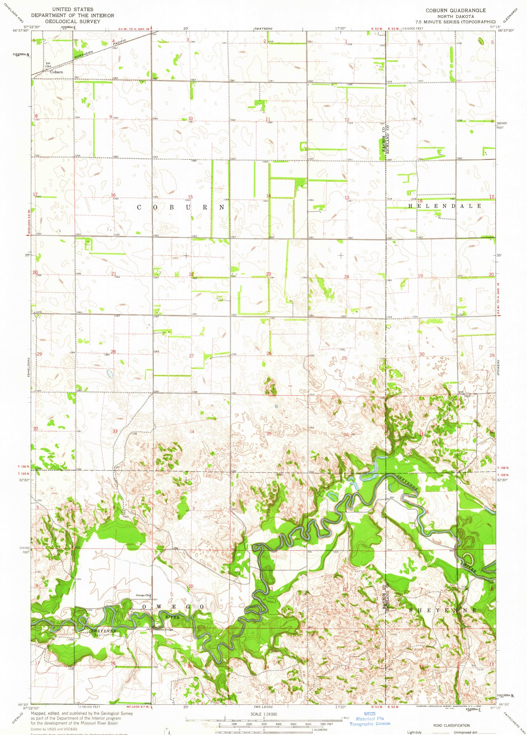
Topography from aerial photographs by photogrammetric methods and by planetable surveys 1960. Aerial photographs taken 1952 and 1958 Polyconic projection. 1927 North American datum 10,000-foot grid based on North Dakota coordinate system, south zone • 1000-meter Universal Transverse Mercator grid ticks, zone 14, shown in blue
