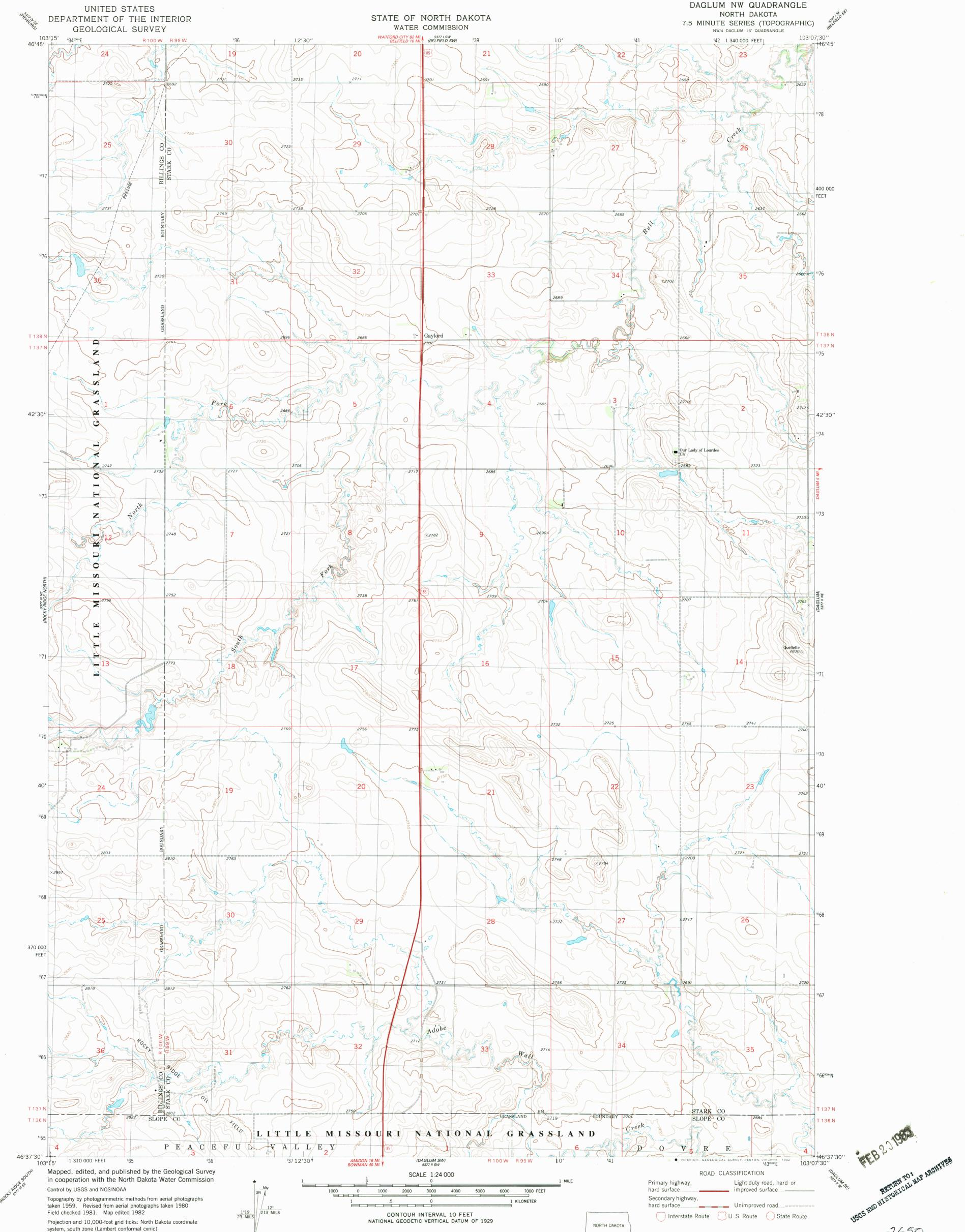
Projection and 10,000-foot grid ticks: North Dakota coordinate system, south zone (Lambert conformal conic) 1000-meter Universal Transverse Mercator grid, zone 13 1927 North American Datum To place on the predicted North American Datum 1983 move the projection lines 4 meters north and 38 meters east as shown by dashed corner ticks
