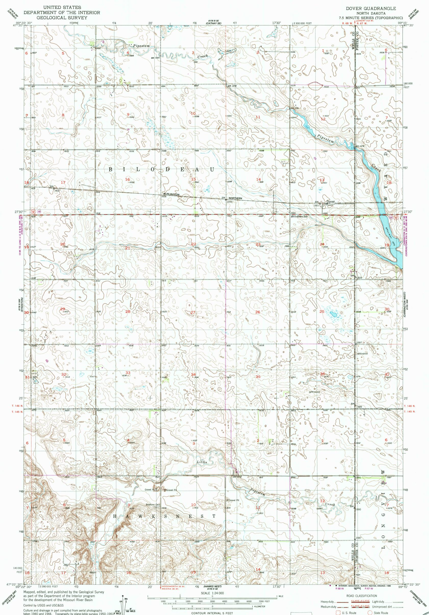
taken 1940 and 1944. Topography by plane-table surveys 1950–1951<sup>4</sup> MILS Polyconic projection. 1927 North American datum 10,000-foot grid based on North Dakota coordinate system, north zone 1000-meter Universal Transverse Mercator grid, zone 14 To place on the predicted North American Datum 1983, move the projection lines 4 meters north and 30 meters east as shown by dashed corner ticks
