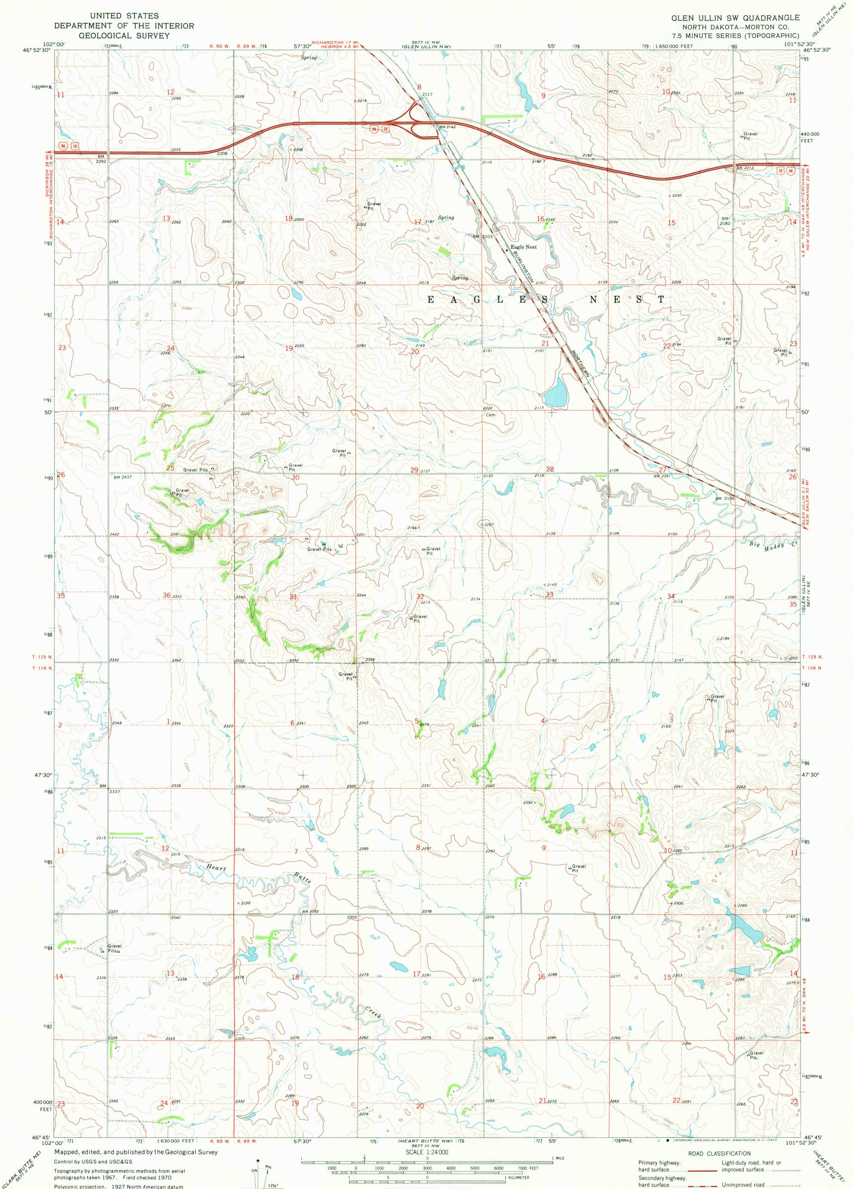
Polyconic projection. 1927 North American datum 10,000-foot grid based on North Dakota coordinate system, south zone 1000-meter Universal Transverse Mercator grid ticks, zone 14, shown in blue
