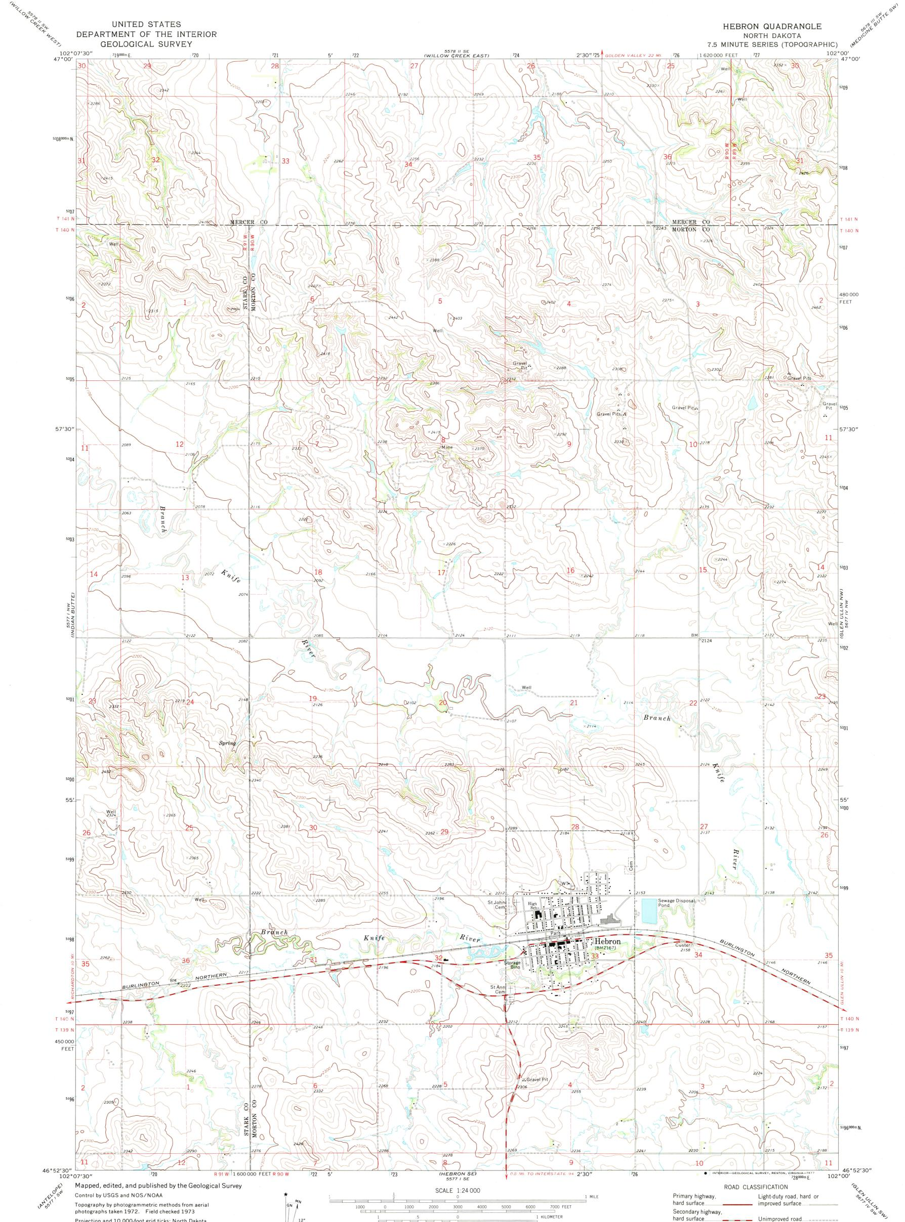
Projection and 10,000-foot grid ticks: North Dakota coordinate system, south zone (Lambert conformal conic) 1000-meter Universal Transverse Mercator grid ticks, zone 13, shown in blue. 1927 North American datum
