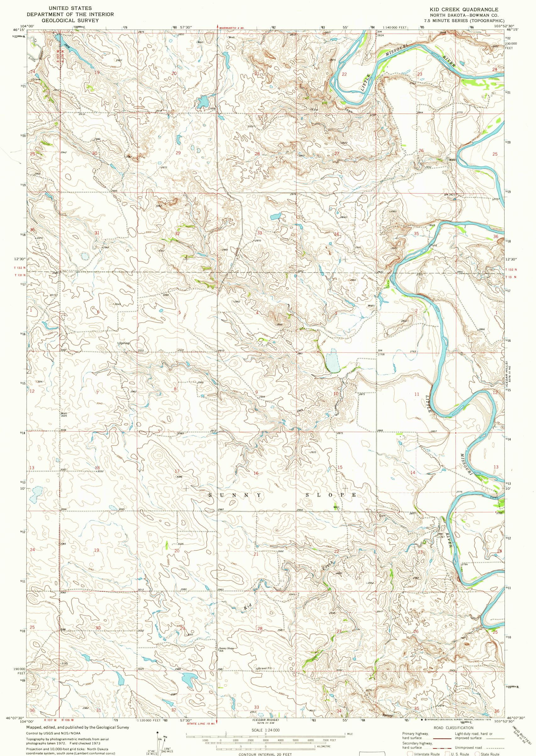
Projection and 10,000-foot grid ticks: North Dakota coordinate system, south zone (Lambert conformal conic) 1000-metre Universal Transverse Mercator grid ticks, zone 13, shown in blue. 1927 North American datum
