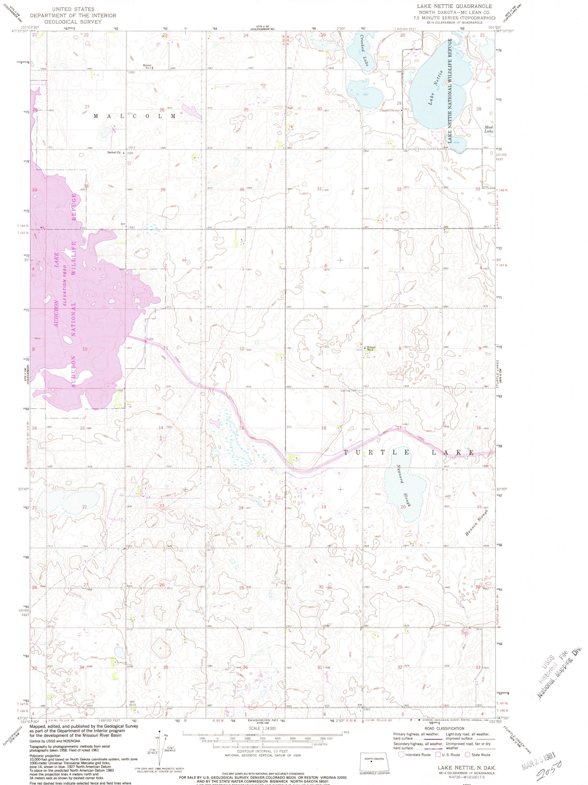
Polyconic projection 10,000-foot grid based on North Dakota coordinate system, north zone 1000-meter Universal Transverse Mercator grid ticks, zone 14, shown in blue. 1927 North American Datum To place on the predicted North American Datum 1983 move the projection lines 4 meters north and 34 meters east as shown by dashed corner ticks
