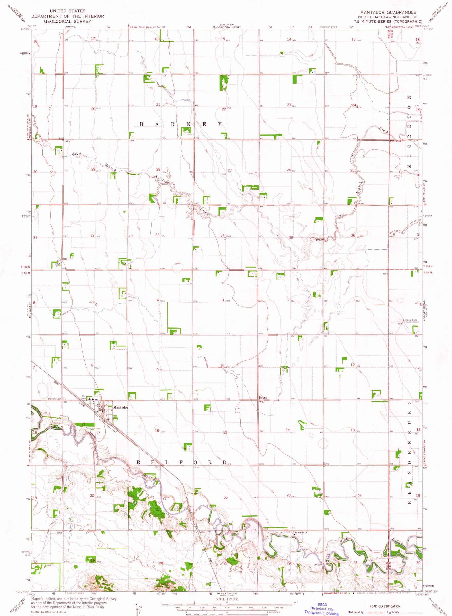
Topography by photogrammetric methods from aerial photographs taken 1963 and planetable surveys 1964
