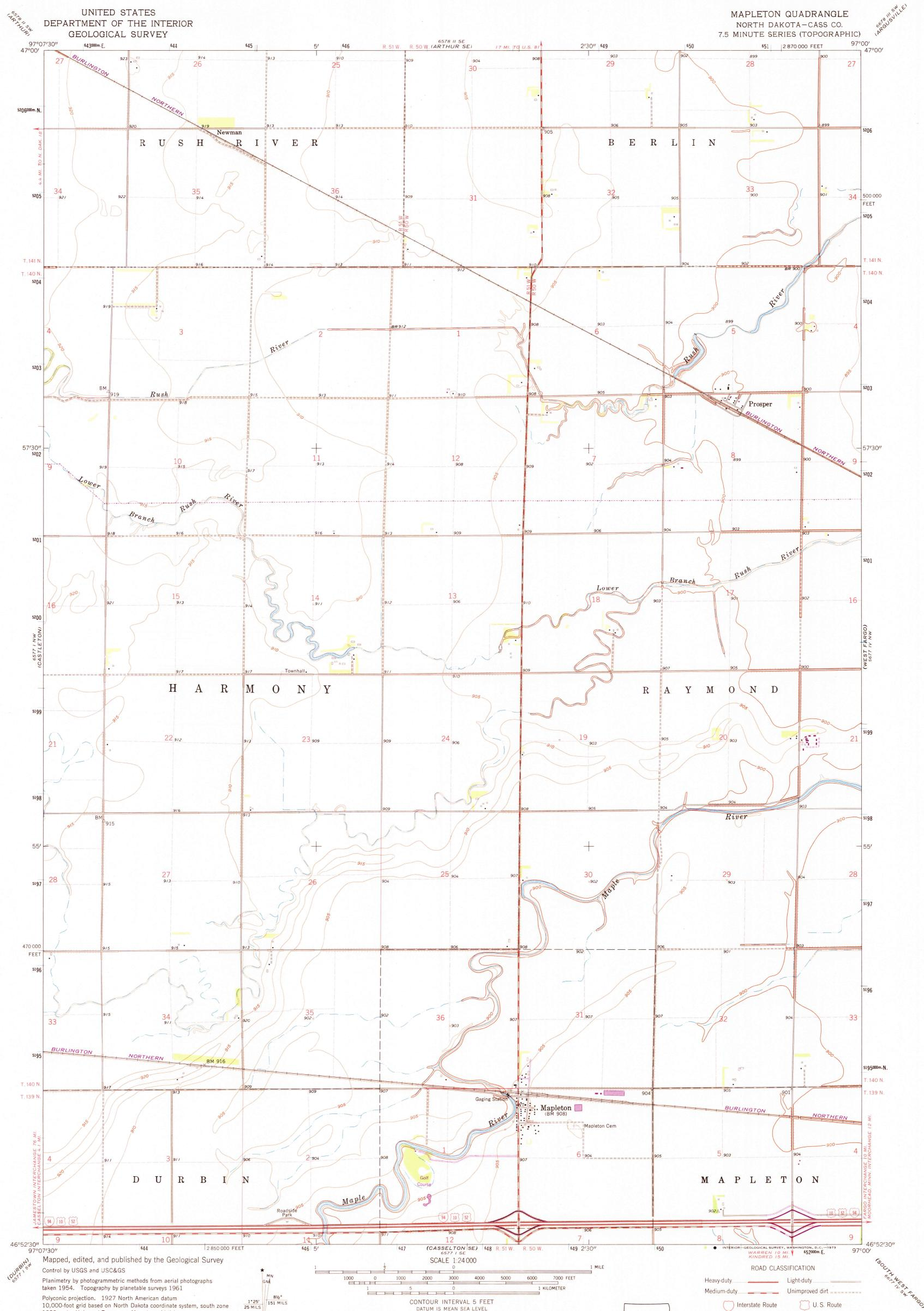
10,000-foot grid based on North Dakota coordinate system, south zone 1000-meter Universal Transverse Mercator grid ticks, zone 14, shown in blue Zone 14, snown in one Fine red dashed lines indicate selected fence and field lines where Conerally visible on aerial photographs This information is unchecked Revisions shown in purple compiled from aerial photographs taken 1971. This information not field checked
