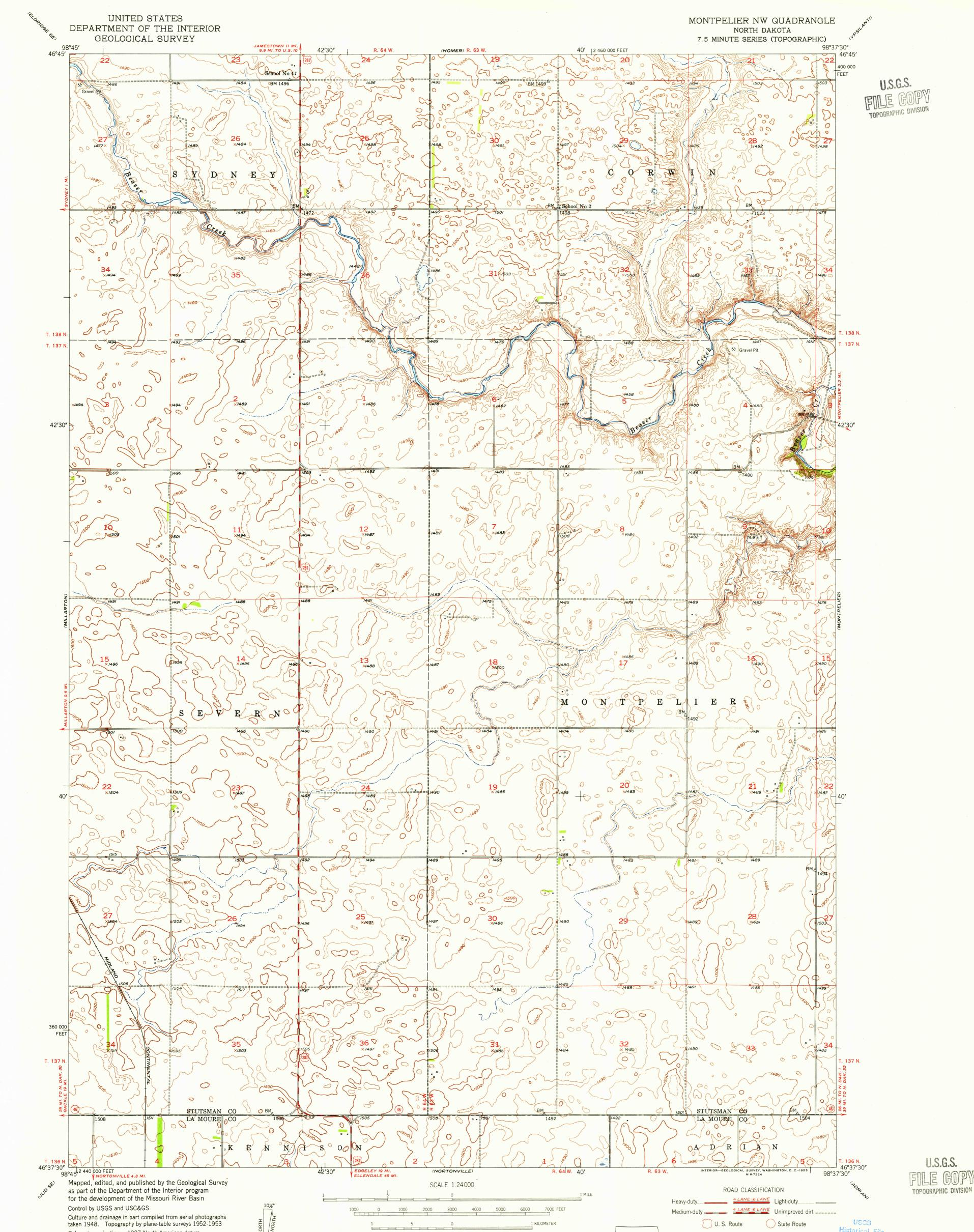
Culture and drainage in part compiled from aerial photographs taken 1948. Topography by plane-table surveys 1952-1953 Polyconic projection. 1927 North American datum. 10,000-foot grid based on North Dakota coordinate system,
