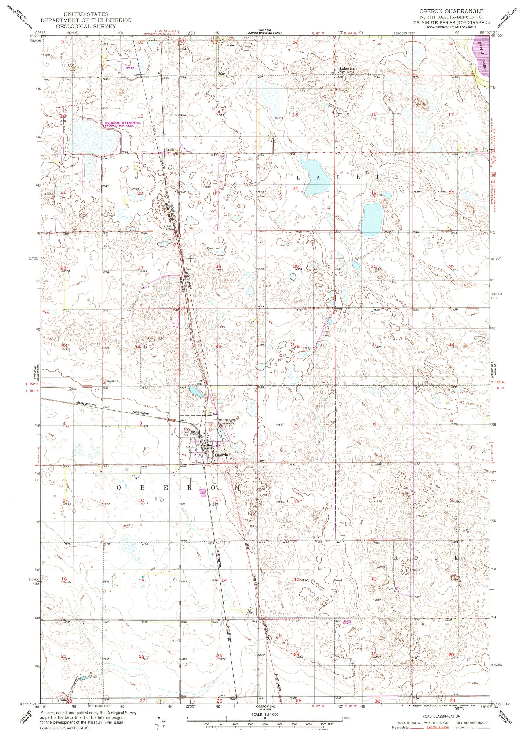
Topography by multiplex methods from aerial photographs taken 1949, and by plane-table surveys 1950 Field check 1950
