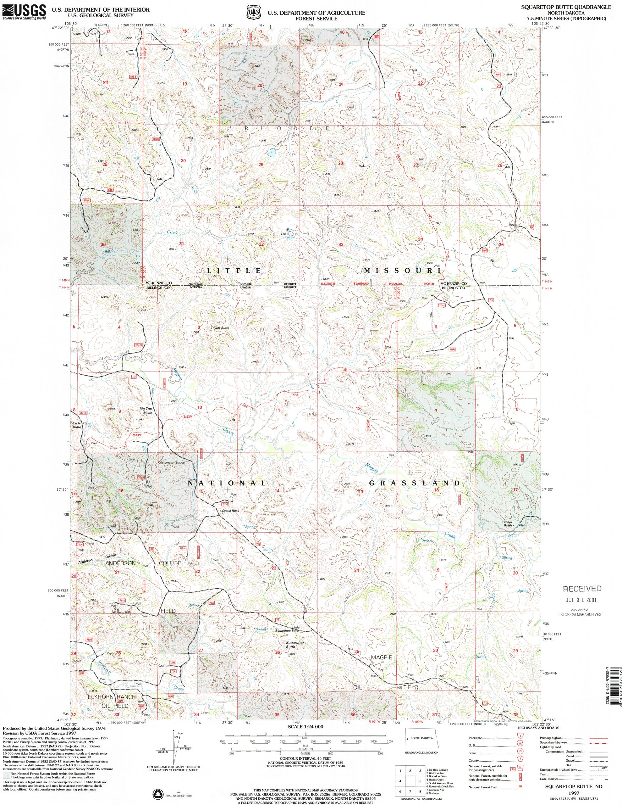
coordinate system, south zone (Lambert conformal conic) 10 000-foot ticks: North Dakota coordinate system, south and north zones Blue 1000-meter Universal Transverse Mercator ticks, zone 13 North American Datum of 1983 (NAD 83) is shown by dashed corner ticks The values of the shift between NAD 27 and NAD 83 for 7.5-minute intersections are obtainable from National Geodetic Survey NADCON software
