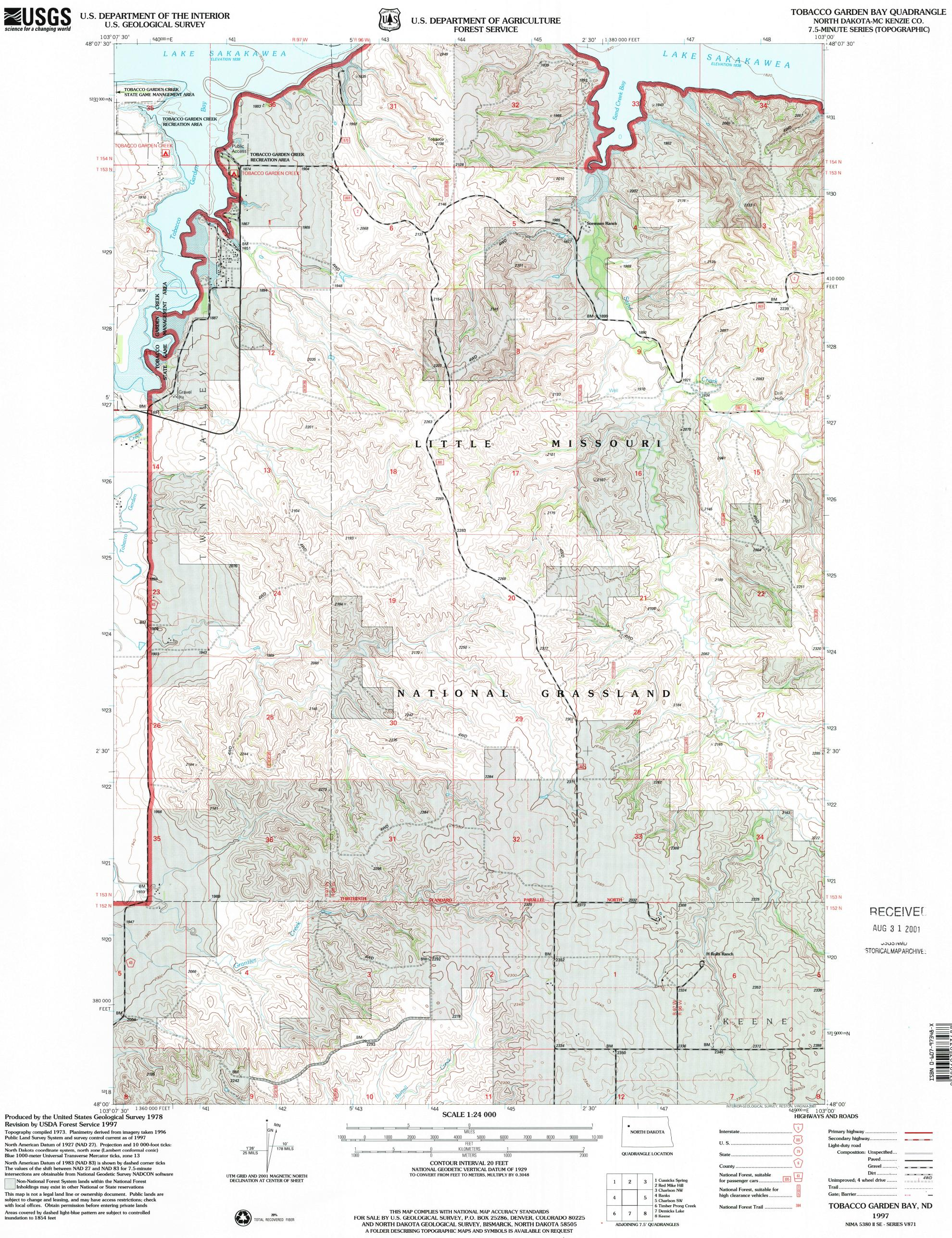
North American Datum of 1927 (NAD 27). Projection and 10 000-foot ticks: North Dakota coordinate system, north zone (Lambert conformal conic) Blue 1000-meter Universal Transverse Mercator ticks, zone 13 North American Datum of 1983 (NAD 83) is shown by dashed corner ticks The values of the shift between NAD 27 and NAD 83 for 7.5-minute intersections are obtainable from National Geodetic Survey NADCON software
