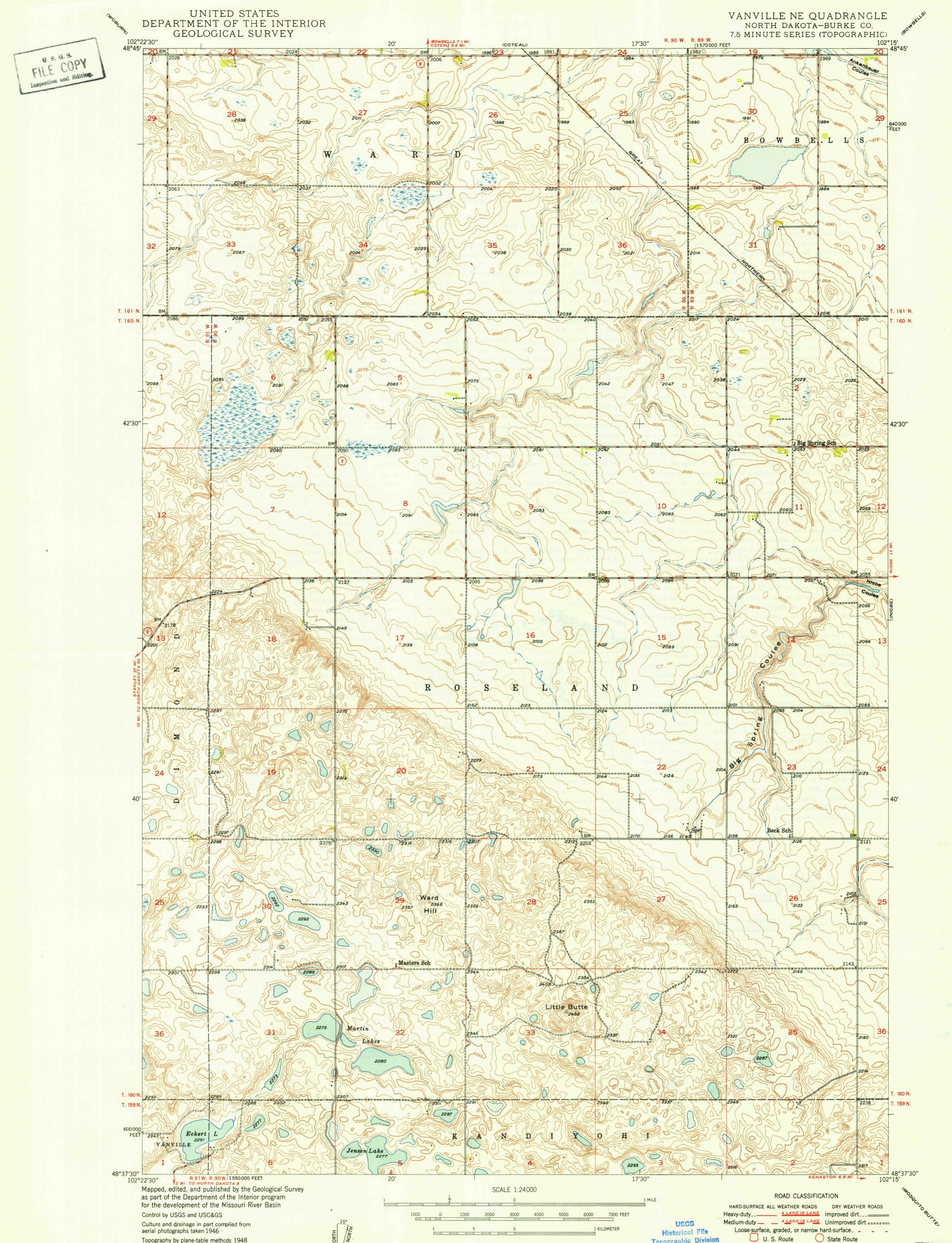
aerial photographs taken 1946 Topography by plane-table methods 1948 Polyconic projection. 1927 North American datum 10,000-foot grid based on North Dakota coordinate system, north zone
