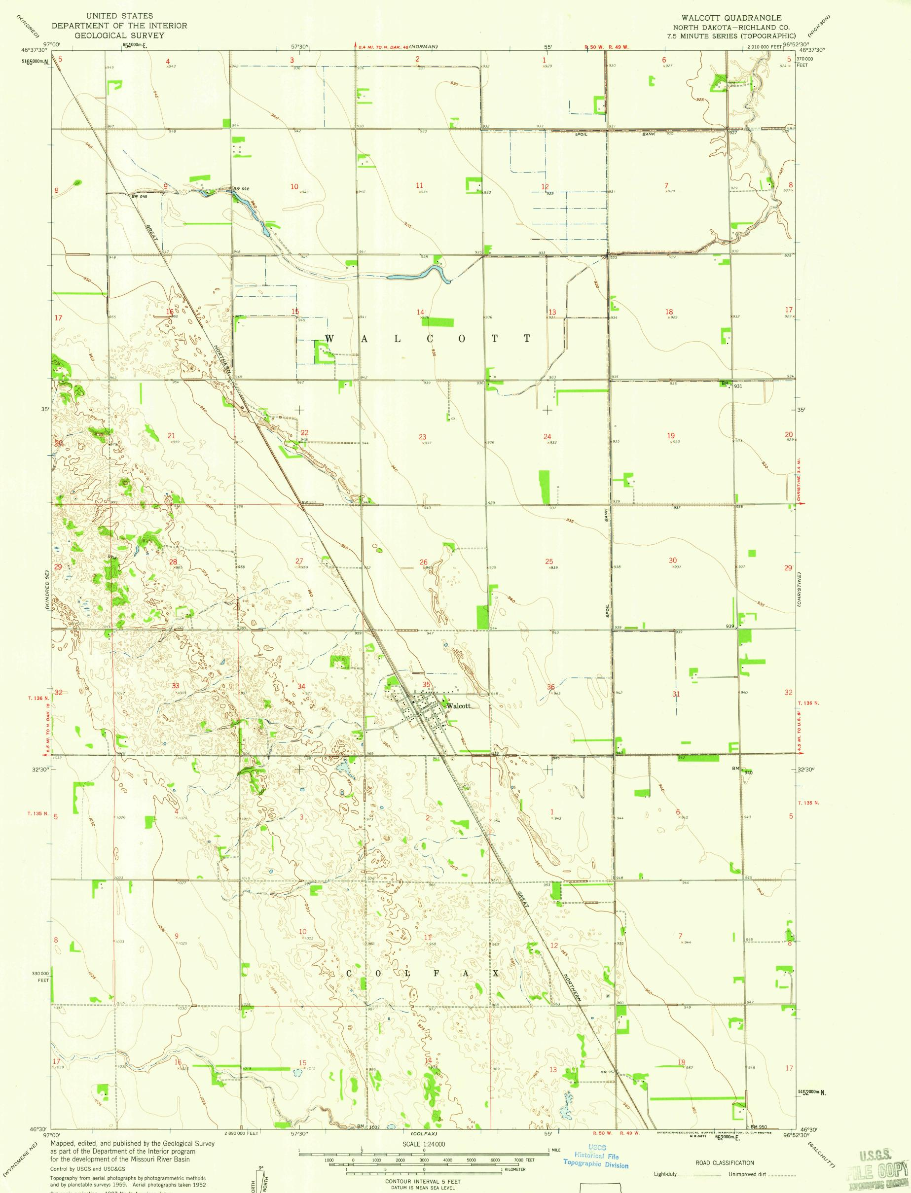
Topography from aerial photographs by photogrammetric methods and by planetable surveys 1959. Aerial photographs taken 1952 Polyconic projection. 1927 North American datum 10,000-foot grid based on North Dakota coordinate system, south zone 1000-meter Universal Transverse Mercator grid ticks, zone 14, shown in blue
