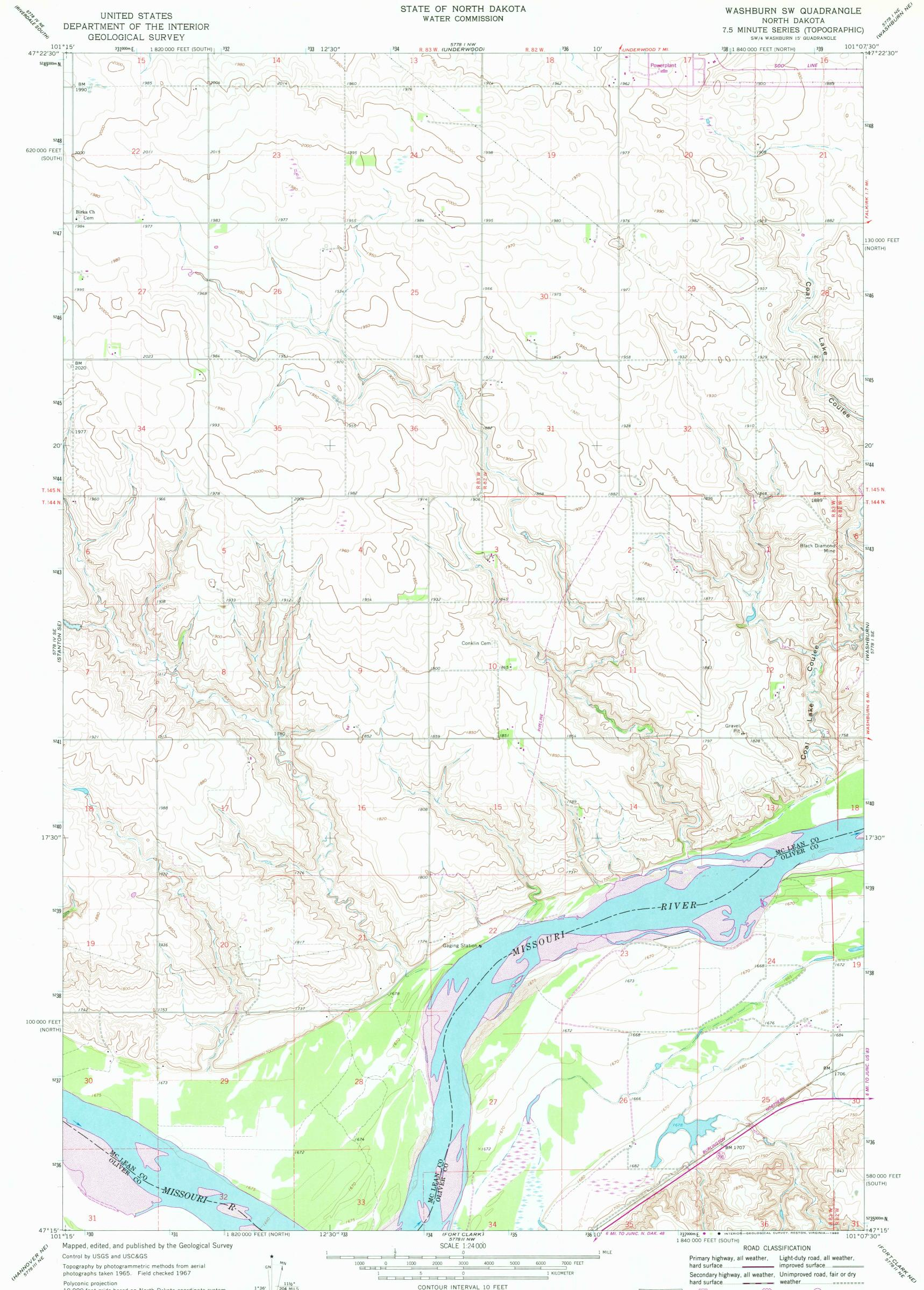
10,000-foot grids based on North Dakota coordinate system, north and south zones 1000-meter Universal Transverse Mercator grid ticks, zone 14, shown in blue 1927 North American Datum To place on the predicted North American Datum 1983 move the projection lines 5 meters north and
