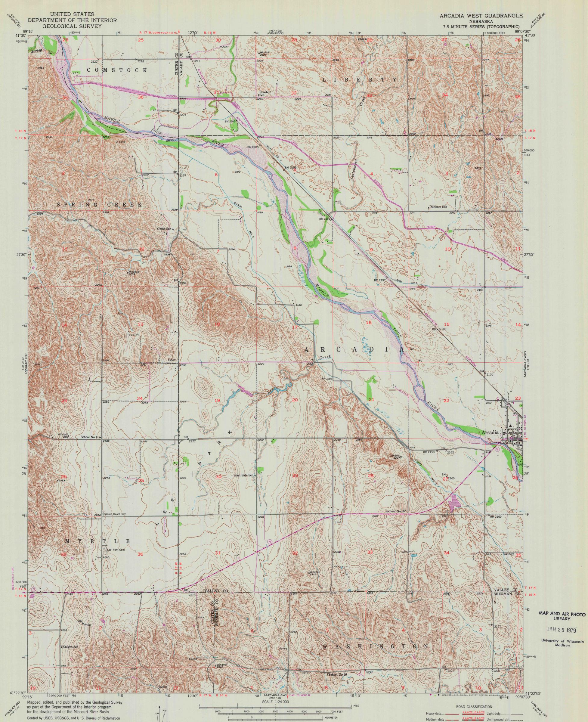
Topography by multiplex methods from aerial photographs taken 1949, by plane-table surveys 1951, and in part by U. S. Bureau of Reclamation. Field check 1951
