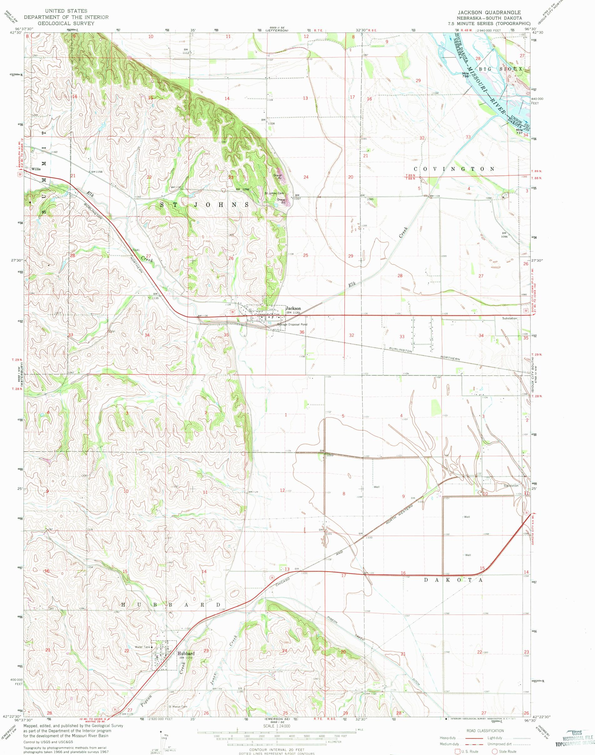
Topography by photogrammetric methods from aerial photographs taken 1966 and planetable surveys 1967
