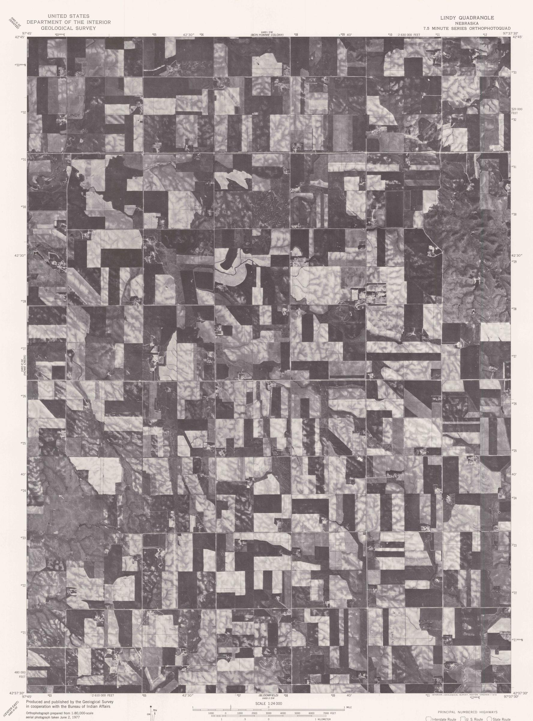
Projection and 10,000-foot grid ticks: Nebraska coordinate system, north zone (Lambert conformal conic) 1000-meter Universal Transverse Mercator grid, zone 14. 1927 North American datum
