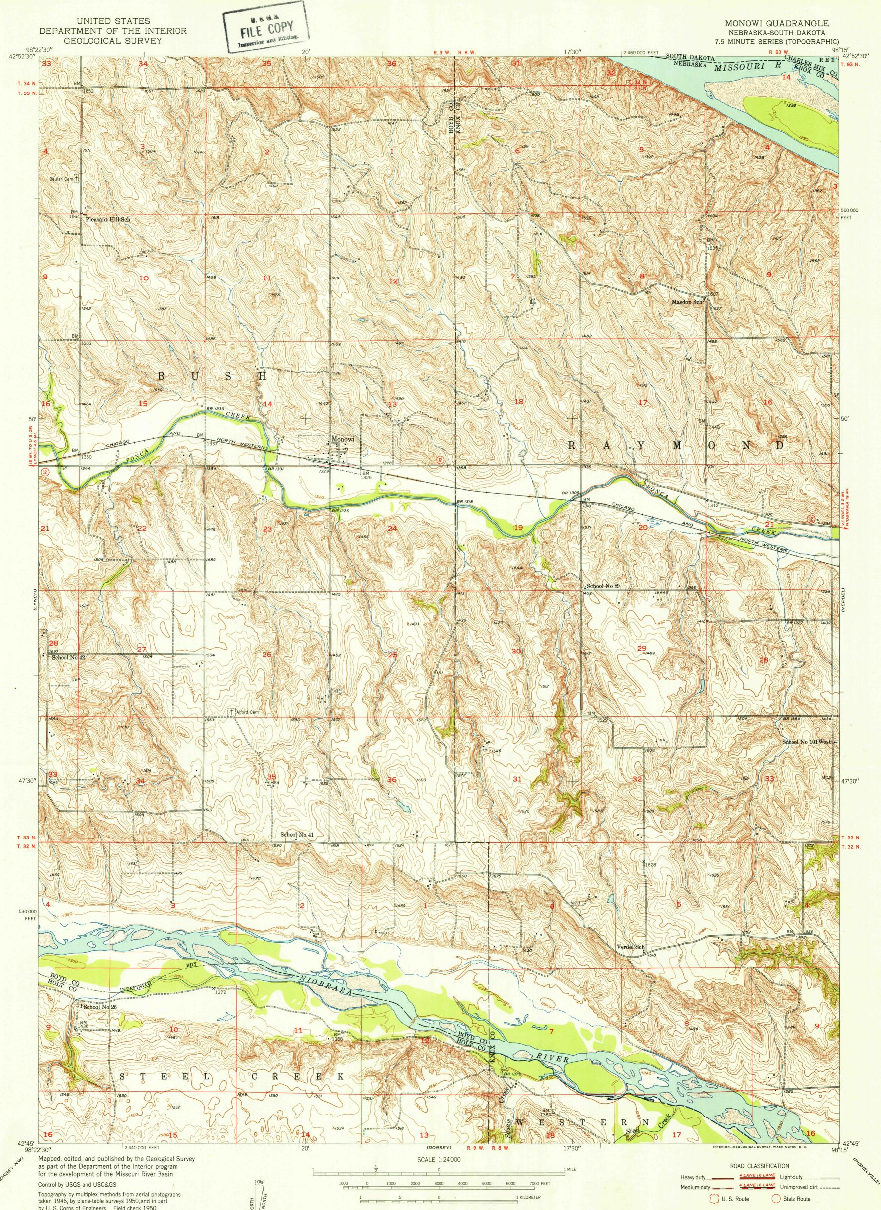
Topography by multiplex methods from aerial photographs taken 1946, by plane-table surveys 1950, and in part by U. S. Corps of Engineers. Field check 1950 Polyconic projection. 1927 North American datum 10,000-foot grid based on Nebraska coordinate system,
