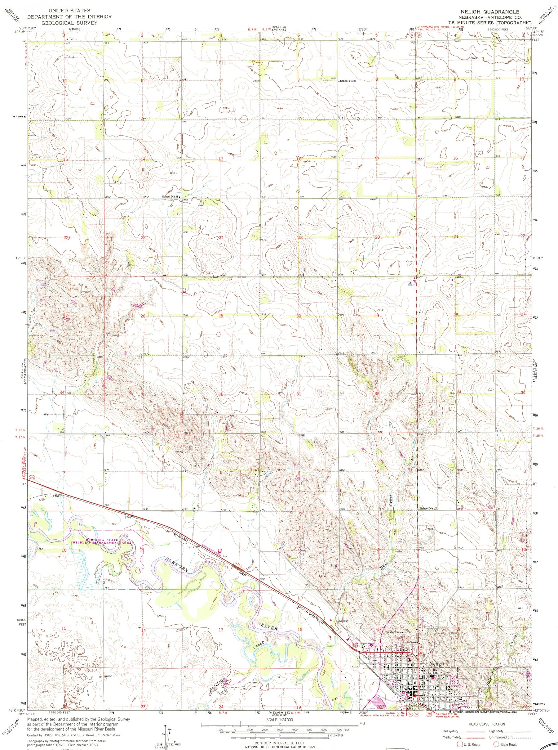
Topography by photogrammetric methods from aerial photographs taken 1961. Field checked 1963 Polyconic projection. 1927 North American datum 10,000-foot grid based on Nebraska coordinate system, north zone 1000-meter Universal Transverse Mercator grid ticks, zone 14, shown in blue
