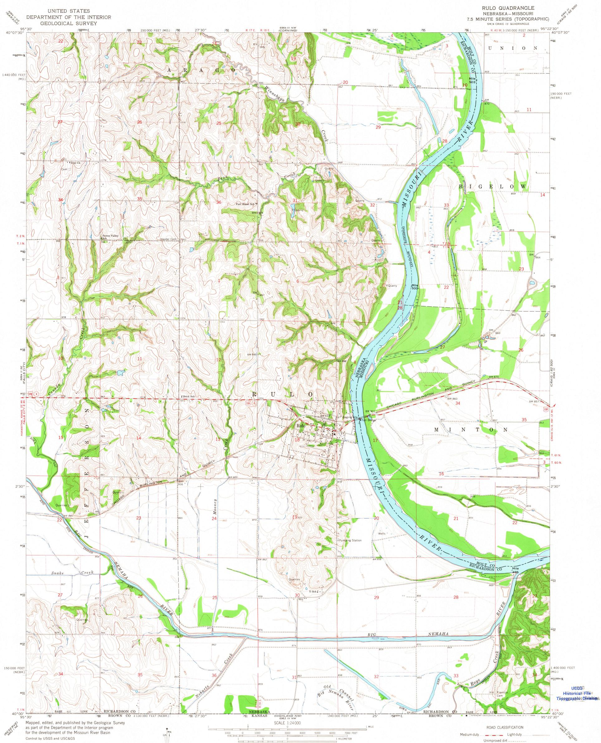
Topography by photogrammetric methods from aerial photographs taken 1963 and planetable surveys 1965
