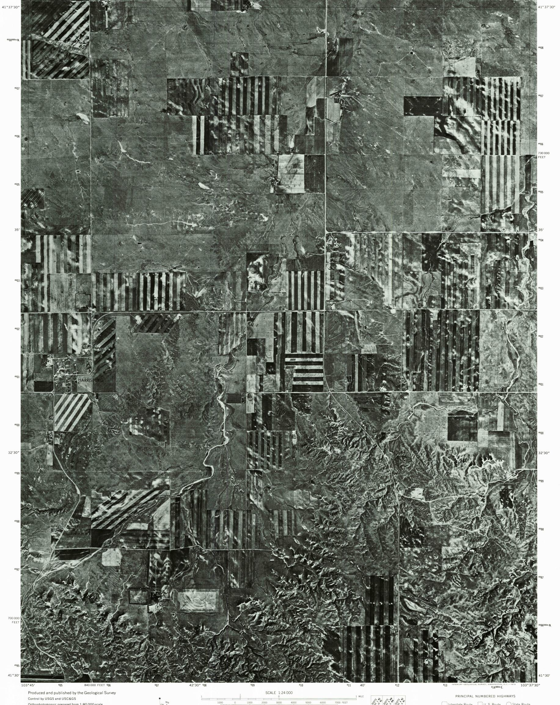
Orthophotomosaic prepared from 1:80 000-scale aerial photographs taken May 3, 1973 Projection and 10,000-foot grid ticks: Nebraska coordinate system, south zone (Lambert conformal conic) 1000-meter Universal Transverse Mercator grid, zone 13. 1927 North American datum Photoimagery transformed by scanning techniques which may produce double or mismatched images; use the mean of image positions for map point
