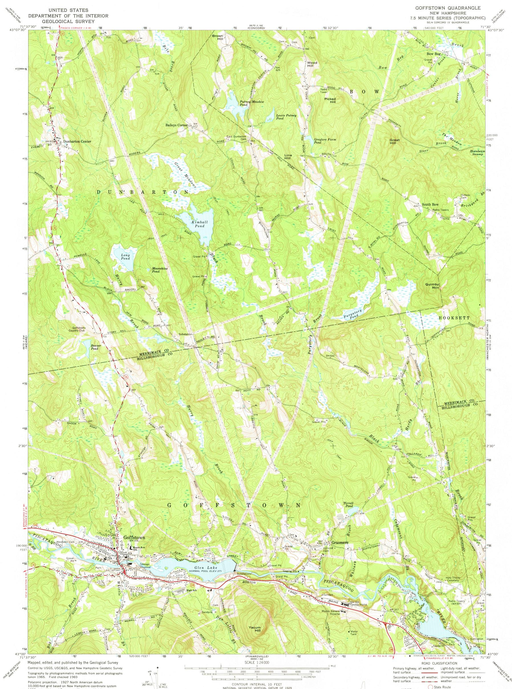
Polyconic projection. 1927 North American datum 10,000-foot grid based on New Hampshire coordinate system 1000-meter Universal Transverse Mercator grid ticks, zone 19, shown in blue
