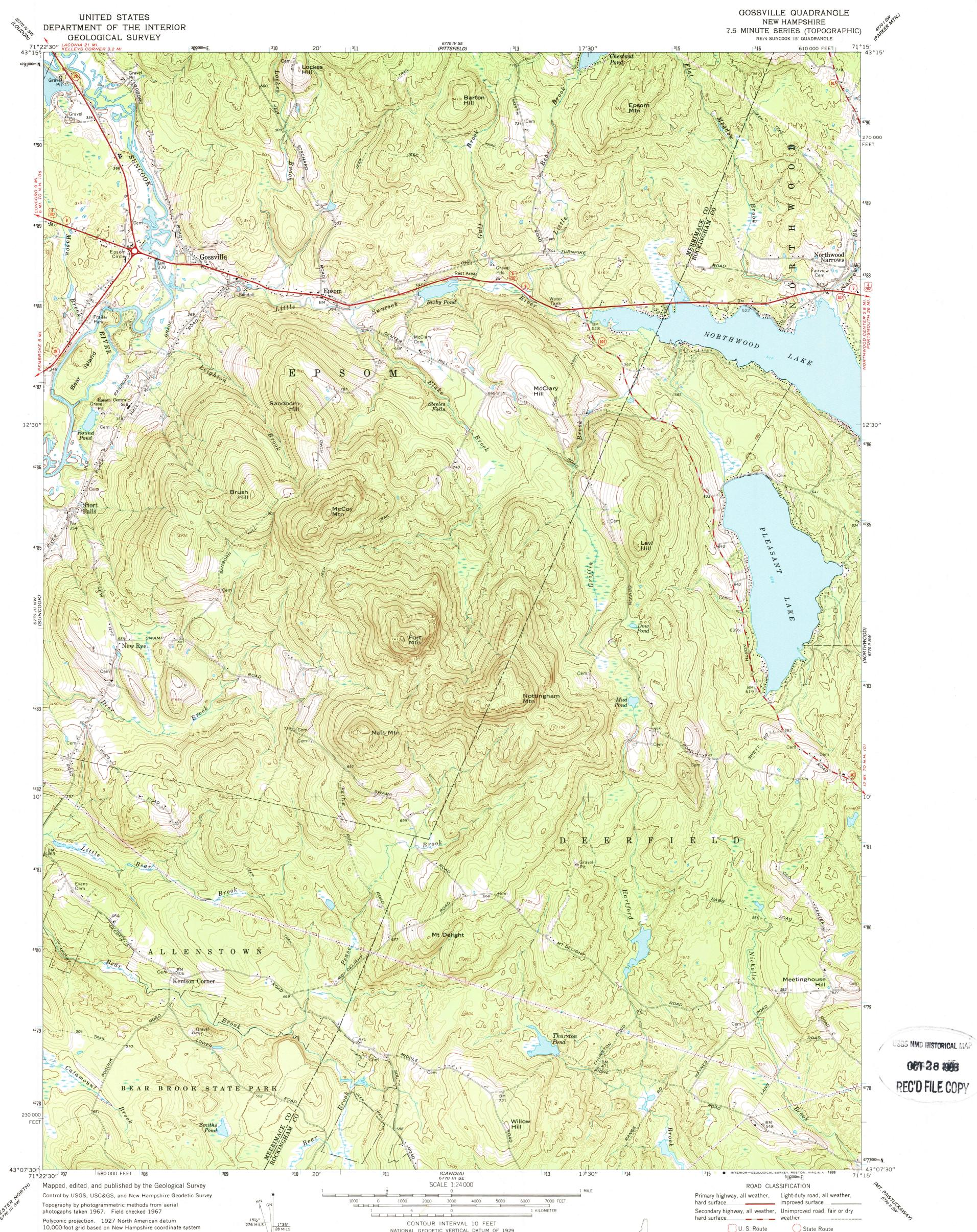
Polyconic projection. 1927 North American datum 10,000-foot grid based on New Hampshire coordinate system 1000-meter Universal Transverse Mercator grid ticks, zone 19, shown in blue
