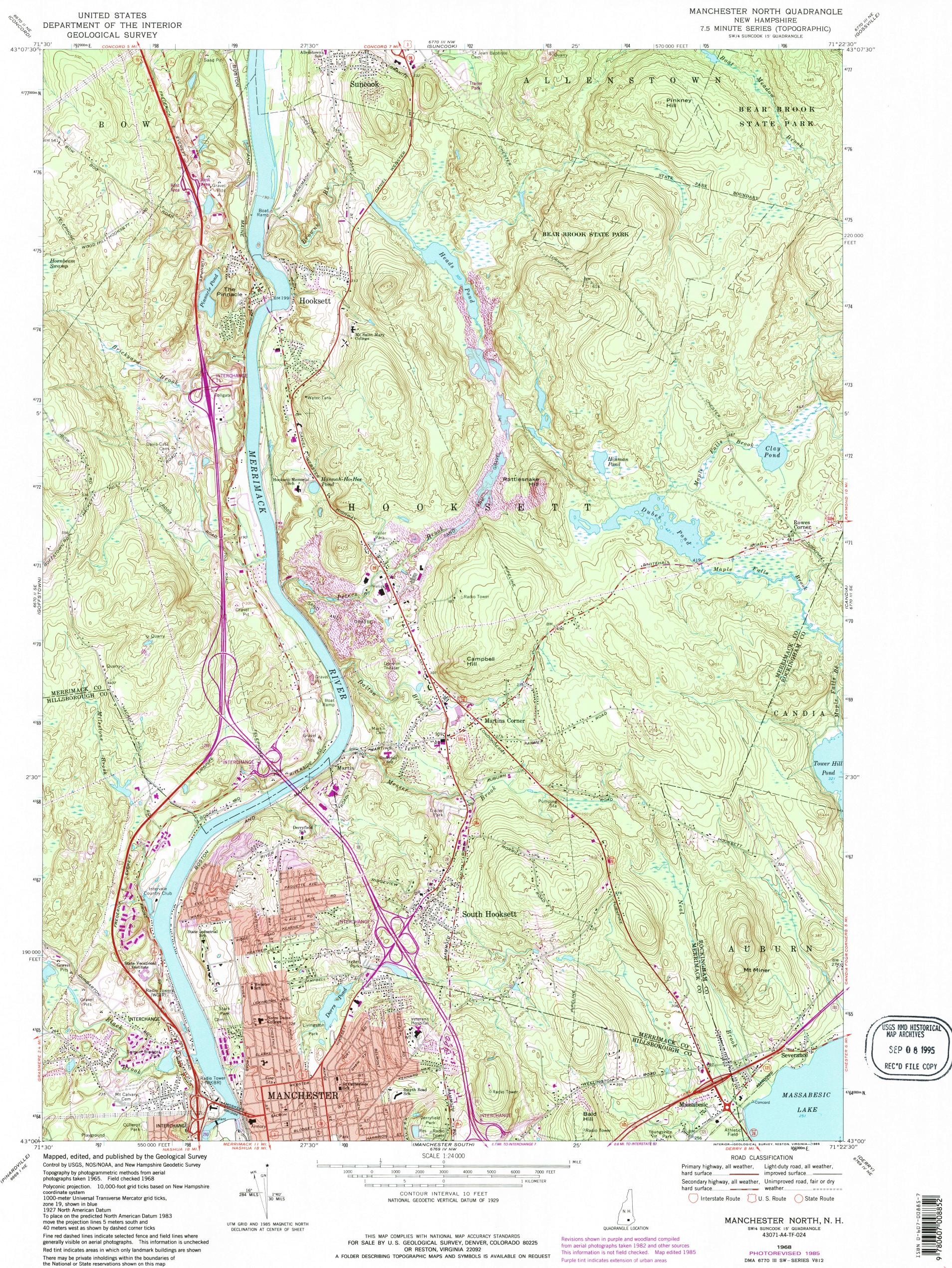
1000-meter Universal Transverse Mercator grid ticks, zone 19, shown in blue 1927 North American Datum To place on the predicted North American Datum 1983 move the projection lines 5 meters south and 40 meters west as shown by dashed corner ticks
