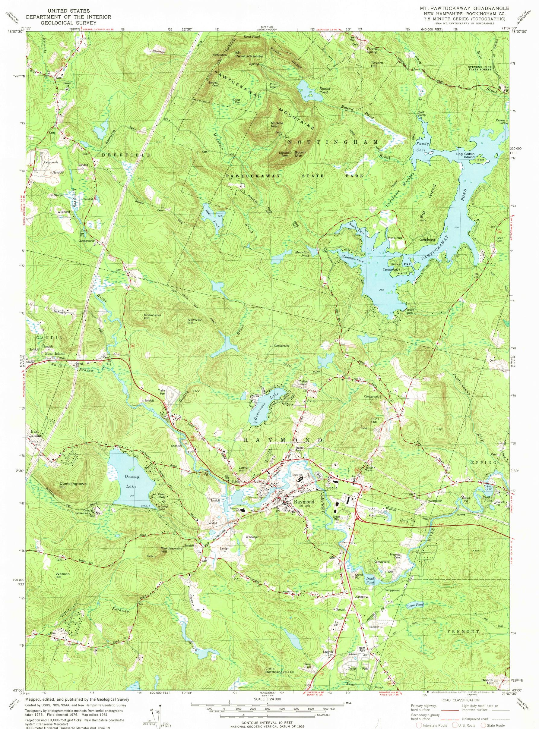
Projection and 10,000-foot grid ticks: New Hampshire coordinate system (transverse Mercator) 1000-meter Universal Transverse Mercator grid, zone 19 1927 North American Datum To place on the predicted North American Datum 1983 move the projection lines 6 meters south and 41 meters west as shown by dashed corner ticks
